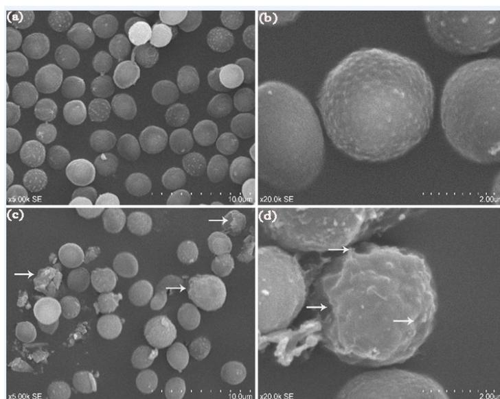
**Figure 6.** SEM of *P. expansum*. *P. expansum* conidia treated with distilled water (a,b), or BanTLP at 60  $\mu\text{M}$  (c,d) for 12 h. Arrows refer to the morphologic alterations in conidia, such as collapsed cell wall and severe contraction (magnification  $\times 5000$ , and 20,000).
