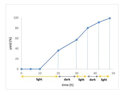
**Figure 1.** Light-dark cycle experiment with N-[(pentyl-2-carbonyl)oxy]phthalimide (0.3 mmol), isoquinoline (0.2 mmol) and *p*-toluenesulfonic acid (0.3 mmol) in DMF (0.1 M). The reaction mixture was irradiated for certain times with a 100 W blue LED module (emission spectra see Supporting Information, Figure S2) and the yield was determined by NMR spectroscopy with 1,4-bis-(trimethylsilyl)benzene as an internal standard.
