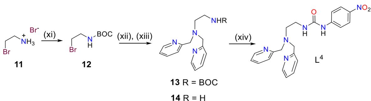
**Scheme 2.** Synthesis of ligand L<sup>4</sup>: (xi) di-*tert*-butyl dicarbonate, dioxane, 0 °C, 48 h, 80% (**12**); (xii) Bis(pyridin-2-ylmethyl)amine, CH<sub>3</sub>CN, DIPEA, 70 °C, 3 d, 39%; (xiii) trifluoroacetic acid (TFA:CH<sub>2</sub>Cl<sub>2</sub> (1:1), r.t., 16 h, 96%; (xiv) 1-isocyanato-4-nitrobenzene, CHCl<sub>3</sub>, r.t., 2 h, 85%.
