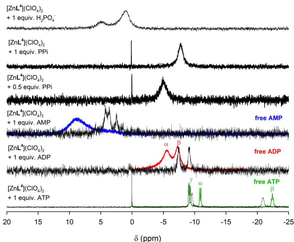
**Figure 7.**  $^{31}\text{P}$  NMR spectra (500 MHz, 298 K) recorded for  $[\text{ZnL}^4]^{2+}$  complex in the presence of AMP, ADP, ATP and phosphate as their sodium salts in  $\text{dms}\text{-}d_6$ . The  $^{31}\text{P}$  NMR spectra of free metabolites are shown as colored traces.
