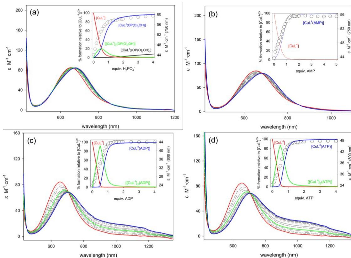
**Figure 4.** Family of UV/vis spectra taken during the course of the titration of  $[\text{CuL}^4]^{2+}$  ( $5 \times 10^{-3}$  M in  $\text{H}_2\text{O}$ , pH 7.0, MOPS 0.1 M, 25 °C) with standard solutions (0.5 M) of: (a)  $\text{NaH}_2\text{PO}_4$ ; (b)  $\text{Na}_2\text{AMP}$ ; (c)  $\text{Na}_2\text{ADP}$ ; and, (d)  $\text{Na}_2\text{ATP}$ . Insets: titration profiles at selected wavelengths vs equivalents of anion and species distribution diagram.
