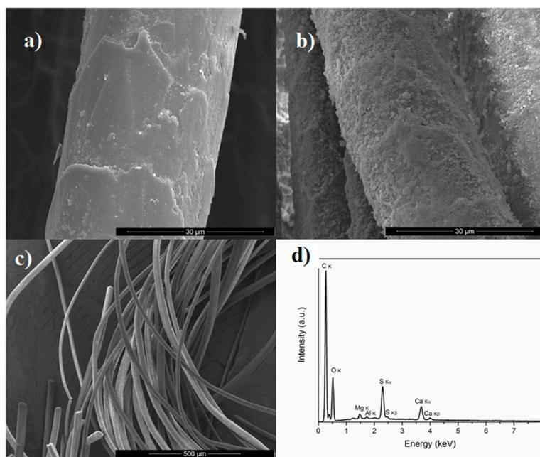
**Figure 2.** Scanning Electron Microscopy (SEM) micrographs of: (a) fibre F1 (magnitude 2500 $\times$ ); (b) fibre F11 (magnitude 2500 $\times$ ); (c) fibre F1 (magnitude 100 $\times$ ); (d) Scanning Electron Microscopy-Energy Dispersive Spectroscopy (SEM-EDS) spectrum of fibre F1.
