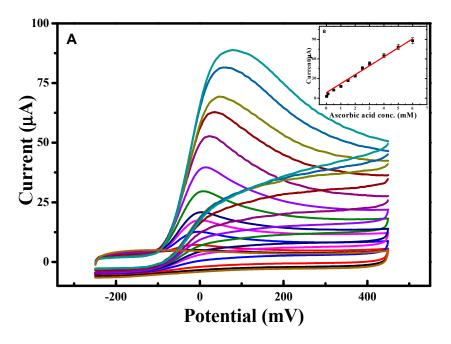
**Figure 8.** (**A**) CVs obtained at various concentrations of ascorbic acid prepared in PBS, pH 7.0 at scan rate of 10 mV/s; and (**B**) calibration plot showing concentration of ascorbic acid prepared in PBS, pH 7.0 at scan rate of 10 mV/s.
