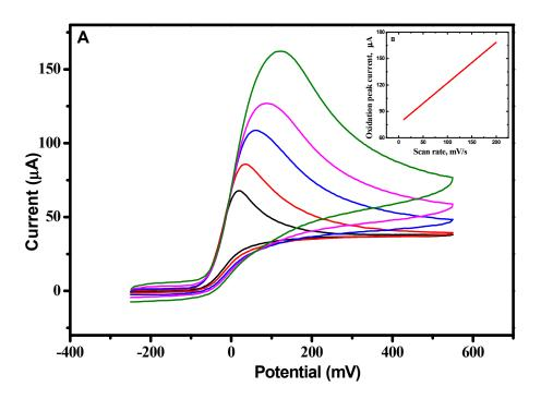
**Figure 7.** (**A**) CVs were obtained at a RSNMC/GC electrode in 3 mM Ascorbic acid prepared in PBS, pH 7.0 at 10, 20, 50, 100, and 200 mV/s scan rates; and (**B**) relationship between peak current and scan rate.
