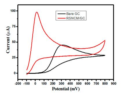
**Figure 6.** CVs obtained for RSNMC/GC and bare GC in 3 mM ascorbic acid prepared in PBS, pH 7.0 at scan rate of 20 mV/s.
