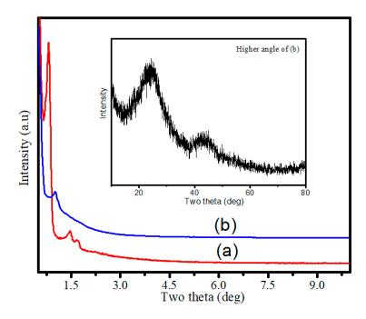
**Figure 2.** (a) XRD patterns of calcined SBA-15 silica template and (b) the rice starch-based nano/mesoporous carbon (RSNMC). The inset shows the higher angle XRD pattern of the RSNMC.
