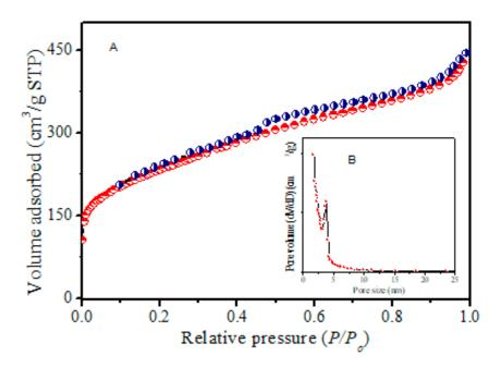
**Figure 4.** (**A**) N<sub>2</sub> isotherms of rice starch-based mesoporous carbon RSNMC; (**B**) The inset shows the pore size distribution of RSNMC.
