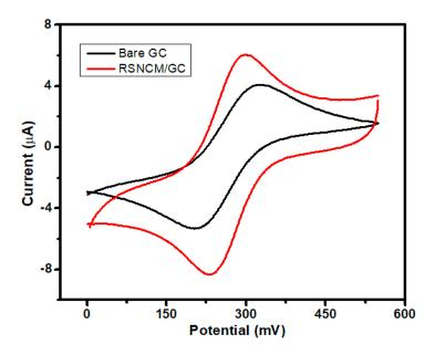
**Figure 5.** CVs obtained for a RSNMC/ glassy carbon (GC) and bare GC electrode in  $1.0 \text{ mM K}_3\text{Fe}(\text{CN})_6$  prepared in PBS, pH 7.0 at scan rate of 20 mV/s.
