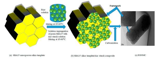
Figure 1. Preparation of nano/mesoporous carbon nanomaterials from rice starch.
