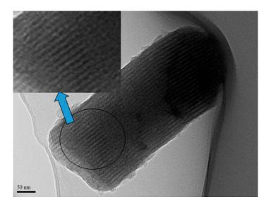
Figure 3. Transmission electron microscope (TEM) image of RSNMC.
