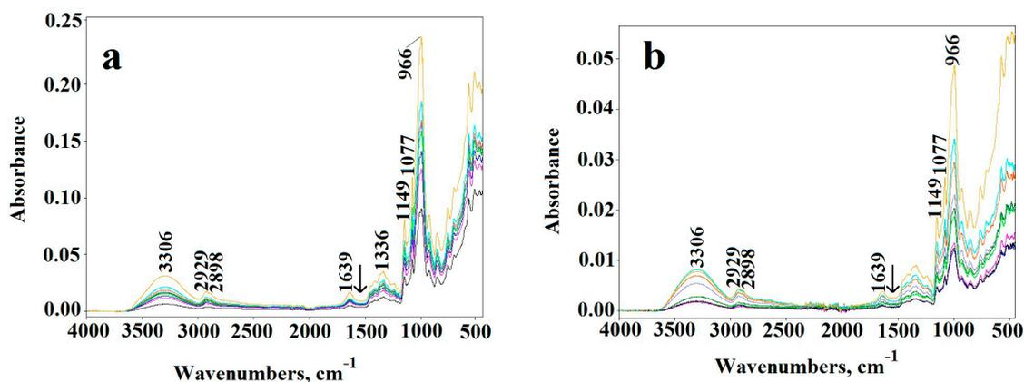
**Figure 2.** The changes in ATR-FTIR spectra of (a) corn starch (CST) and (b) potato starch (PST) after UV-treatment up to 480 min.
