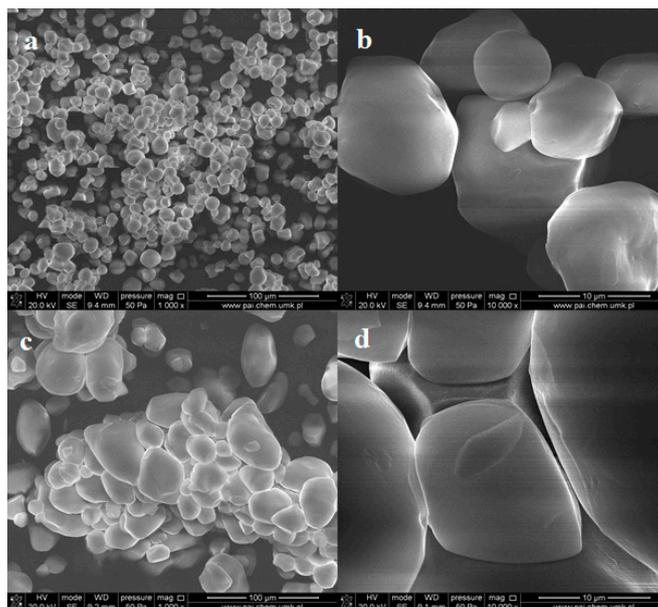
**Figure 1.** SEM images of pristine corn starch (a,b) and potato starch (c,d) in the form of powder at different magnifications.
