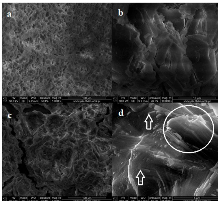
**Figure 9.** SEM images of powder dialdehyde corn starch (a,b) and dialdehyde potato starch (c,d) irradiated 8 h.
