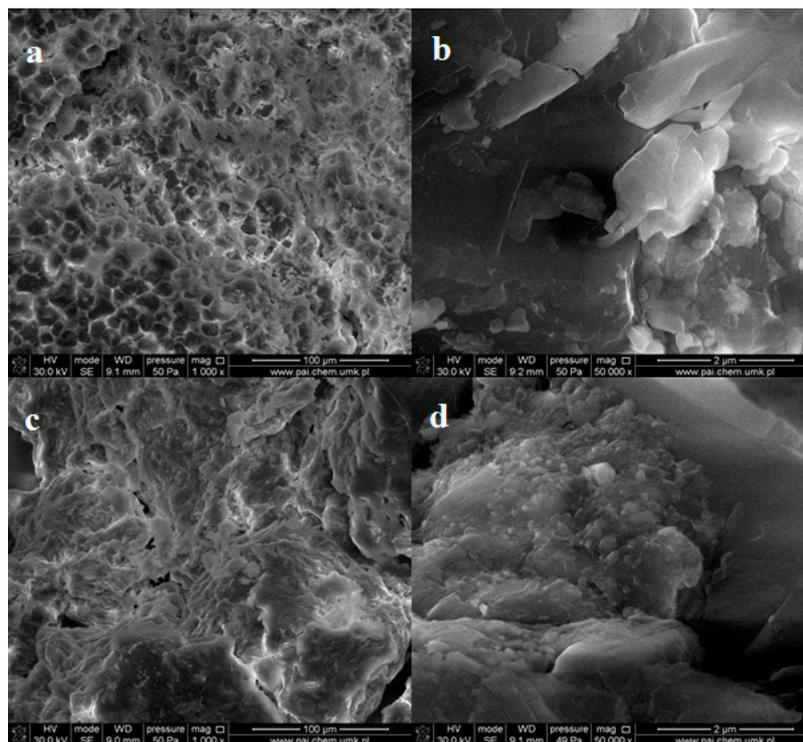
**Figure 4.** SEM images of powder dialdehyde corn starch (a,b) and dialdehyde potato starch (c,d) obtained at 1:0.5 ratio of starch to oxidant.
