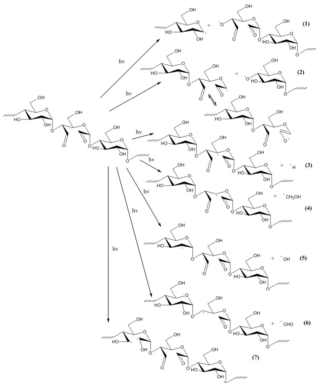
**Figure 12.** Main primary photochemical reactions in the dialdehyde starch (the hydrogen atoms in rings are omitted).
