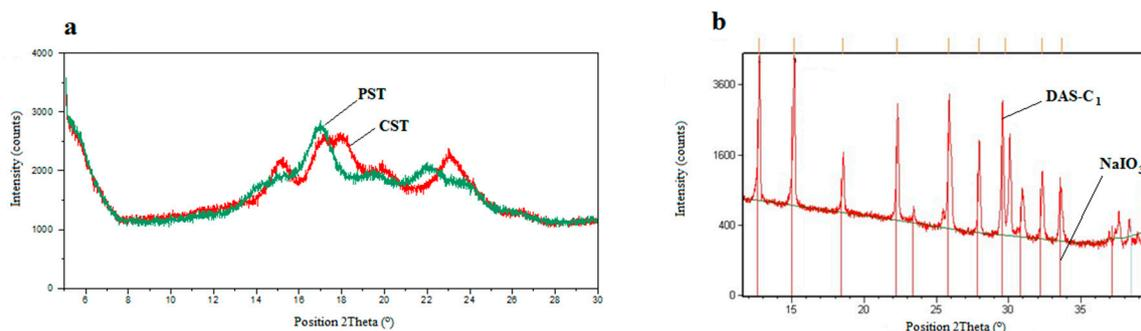
**Figure 10.** X-ray diffraction pattern of the native CST and PST (a), DAS-C with overlapped signals of pure  $\text{NaIO}_3$  hydrate (b).
