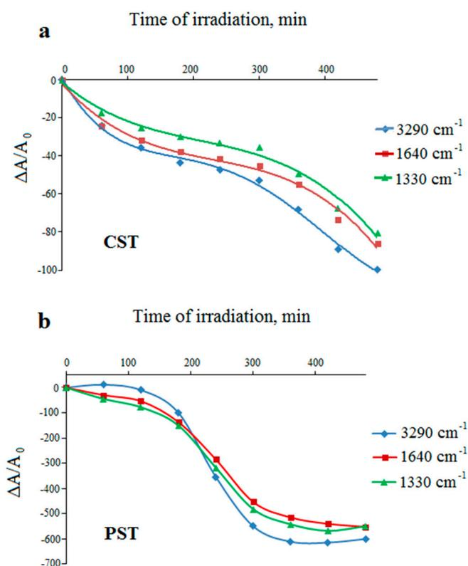
**Figure 7.** Changes in the relative absorbance of the selected bands of UV-irradiated corn (a) and potato (b) starches (unmodified) versus irradiation time.
