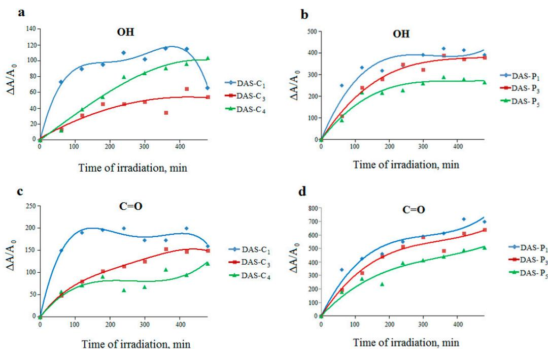
**Figure 8.** Changes in the relative absorbance of hydroxyl (a,b) and carbonyl (c,d) bands for dialdehyde corn starches (DAS-C1, DAS-C3, and DAS-C4) and dialdehyde potato starches (DAS-P1, DAS-P3, and DAS-P5) respectively, versus irradiation time.
