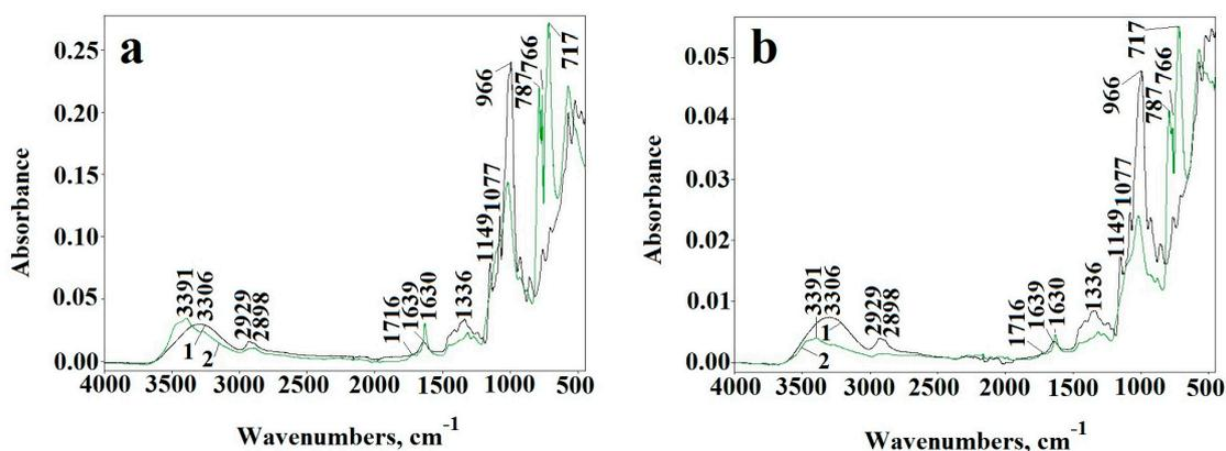
**Figure 5.** ATR-FTIR spectra of corn starch (a) and potato starch (b) (1) and after chemical oxidation to dialdehyde starch (2) and dialdehyde starch (DAS)-C3 (a) and DAS-P3 (b) starch during UV-irradiation for 480 min—arrow indicates the direction of changes after irradiation.
