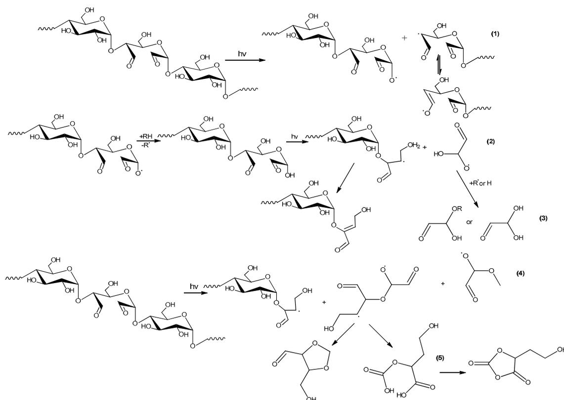
**Figure 14.** Other specific reactions in UV-irradiated the dialdehyde starch.
