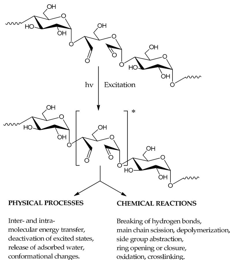
**Figure 11.** Possible photoprocesses in UV-irradiated dialdehyde starch.
