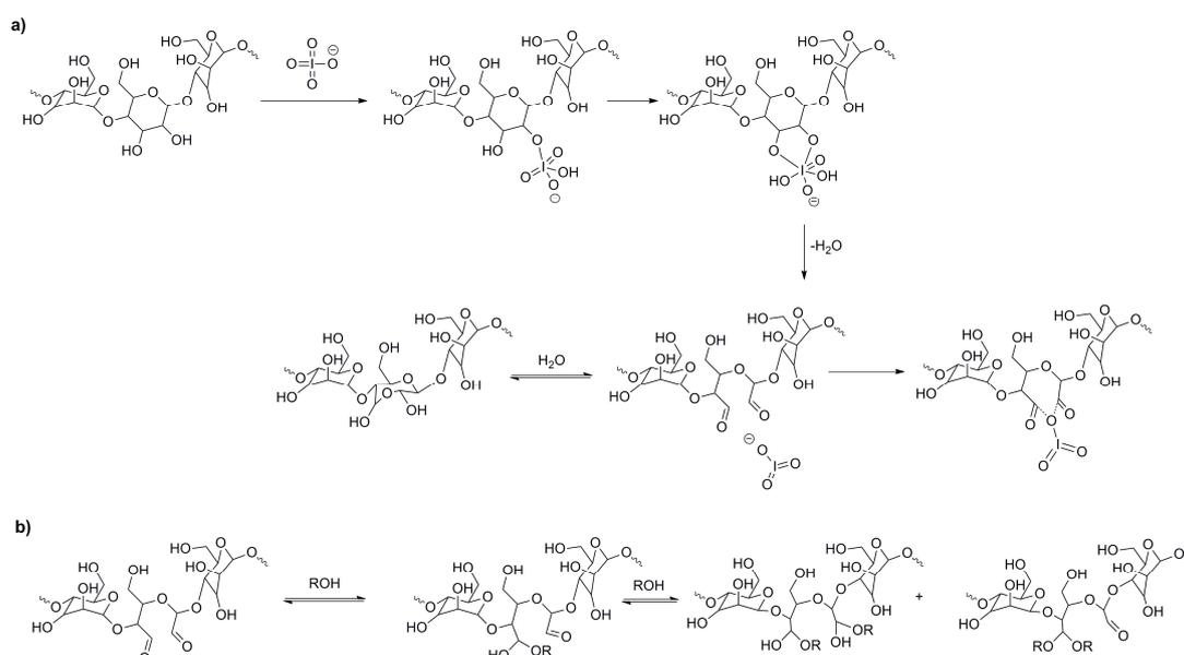
**Figure 3.** Mechanism of starch oxidation with sodium periodate (a), hemiacetals and acetals formation (b).
