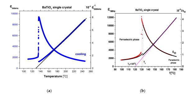
**Figure S1.** Temperature dependence of the real part of the complex permittivity and its inverse shown on the left and right ordinate, respectively, of the (a) SSCG-grown and (b) TSSG-grown BaTiO<sub>3</sub> single crystals. The solid line is the best-fitted result for the inverse dielectric constant in the paraelectric phase obtained by using the Curie–Weiss law. The data of TSSG-grown BaTiO<sub>3</sub> were the modified one reported in Reference 18.
