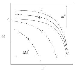
**Figure 11.** Schematic representation of the effect of the parameters of the Turnbull-Fisher equation (Equation (1)) on the temperature dependence of the activation energy (Equation (2)). Arrows show the direction of increase in  $\Delta G^*$  and  $E_D$ . Curves 2 and 3 have the same  $E_D$  as 1, but consecutively increasing values of  $\Delta G^*$ . Curves 4 and 5 have the same  $\Delta G^*$  as 1, but consecutively increasing values of  $E_D$ .
