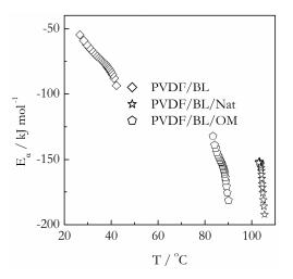
**Figure 10.** Temperature dependence of activation energy for gelation of PVDF/BL in bulk (diamonds) and confined systems PVDF/BL/Nat (stars) and PVDF/BL/OM (pentagons). Confinement is to 9 nm pores.
