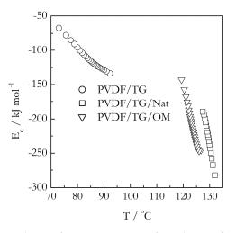
**Figure 9.** Temperature dependence of activation energy for gelation of PVDF/TG in bulk (circles) and confined systems PVDF/TG/Nat (triangles) and PVDF/TG/OM (squares). Confinement is to 9 nm pores.
