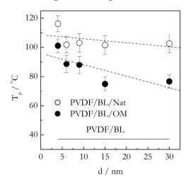
**Figure 7.** DSC peak temperatures for gelation of PVDF/BL in bulk (solid line) and confined systems PVDF/BL/Nat (open circles), PVDF/BL/OM (solid circles) vs. the pore diameter. Dashed line is a guide to the eye.
