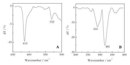
**Figure 1.** FTIR spectra of the bulk PVDF/TG (**A**) and PVDF/BL (**B**) gels. The vertical axis represents the difference in the transmittance between the gel and solvent.
