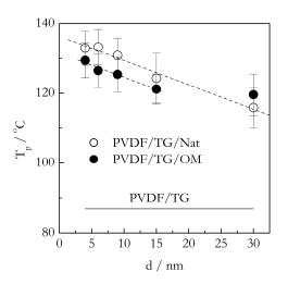
**Figure 5.** DSC peak temperatures for gelation of PVDF/TG bulk (solid line), and confined systems, PVDF/TG/Nat (open circles), PVDF/TG/OM (solid circles) vs. the pore diameter. Dashed line is a guide to the eye.
