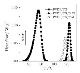
**Figure 3.** DSC curves for TG-based gels at a cooling rate of 8 °C min<sup>-1</sup>. The bulk gel is represented by squares, PVDF/TG/NAT and PVDF/TG/OM gels confined in 9 nm pores represented by solid and open circles, respectively. The heat flow values are given per gram of gel.
