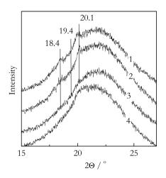
**Figure 2.** X-ray diffractograms of the PVDF nanoconfined gels in 30 nm silica pores: PVDF/TG/NAT (1), PVDF/TG/OM (2) PVDF/BL/NAT (3), and PVDF/BL/OM (4).
