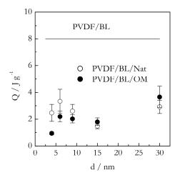
**Figure 8.** Heat of gelation of PVDF/BL in bulk (solid line) and confined systems PVDF/BL/Nat (open circles), PVDF/BL/OM (solid circles) dependence on the pore diameter size. The values of Q are given per gram of gel and represent the average of all cooling rates.
