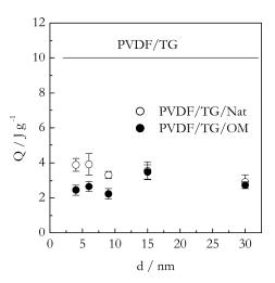
**Figure 6.** Heat of gelation of PVDF/TG in bulk (solid line) and confined systems PVDF/TG/Nat (open circles), PVDF/TG/OM (solid circles) dependence on the pore diameter size. The values of Q are given per gram of gel and represent the average of all cooling rates.
