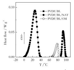
**Figure 4.** DSC curves for BL-based gels at a cooling rate of 8 °C min<sup>-1</sup>. The bulk gel is represented by squares, PVDF/BL/NAT and PVDF/BL/OM gels confined in 9 nm pores represented by solid and open circles, respectively. The heat flow values are given per gram of gel.
