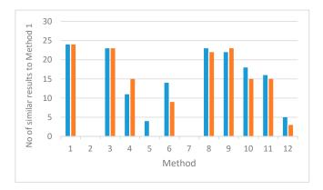
**Figure 4.** Phase 2: Column chart indicating similarity in molecular weight results for 24 heparin samples, between the USP Heparin Sodium monograph method (Method 1) and 11 other distinct chromatographic methods (Table S5). Blue columns plot  $M_w$  data and orange columns plot  $M_{24,000}$ . Data are taken from Table S3A,B; similarity criteria are for  $M_w$ , values differ from Method 1 by less than 500 Da; for  $M_{24,000}$  values differ from Method 1 by less than 10%.
