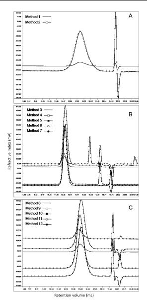
**Figure 3.** Phase 2: Overlay view of USP Heparin Sodium Identification RS chromatographic profiles in 12 distinct chromatographic systems. Panels: (**A**) Methods 1 and 2; (**B**) Methods 3–7; (**C**) Methods 8–12.
