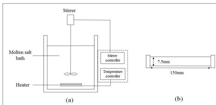
**Figure 4.** (a) Batch fluid extraction system and (b) reactor cell.
