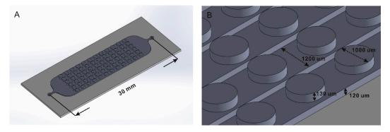
Figure S1. 3D illustration of the SU-8 mold. (A) Full mold; (B) Close-view of the mold.
