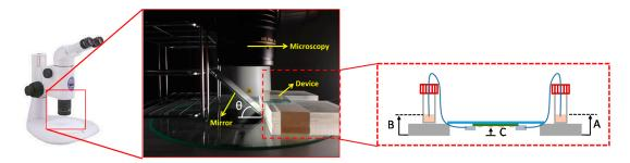
**Figure S2.** Setup of the droplet measurement. **A** and **B** are the combined height of medium and PMMA plate from the microscope stage, whereas C is the distance from the droplet's bottom to the microscope stage.
