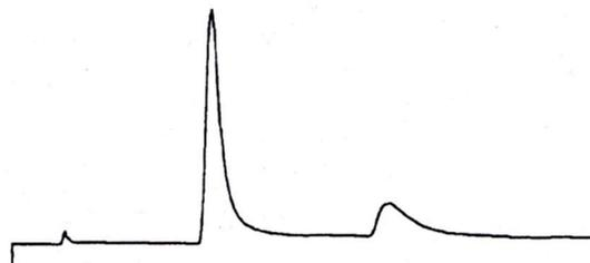
**Figure 17.** HPLC separation of  $C_{60}$  (12.2 min) and  $C_{70}$  (23.5 min) on a Pirkle-type ionically DNBPG containing column (250 × 10 mm I.D.) eluted with *n*-hexane at 5.0 mL/min and detected at 280 nm,  $\alpha = 2.25$  (r.t.). Reprinted with permission from [80]. Copyright (1990) American Chemical Society.
