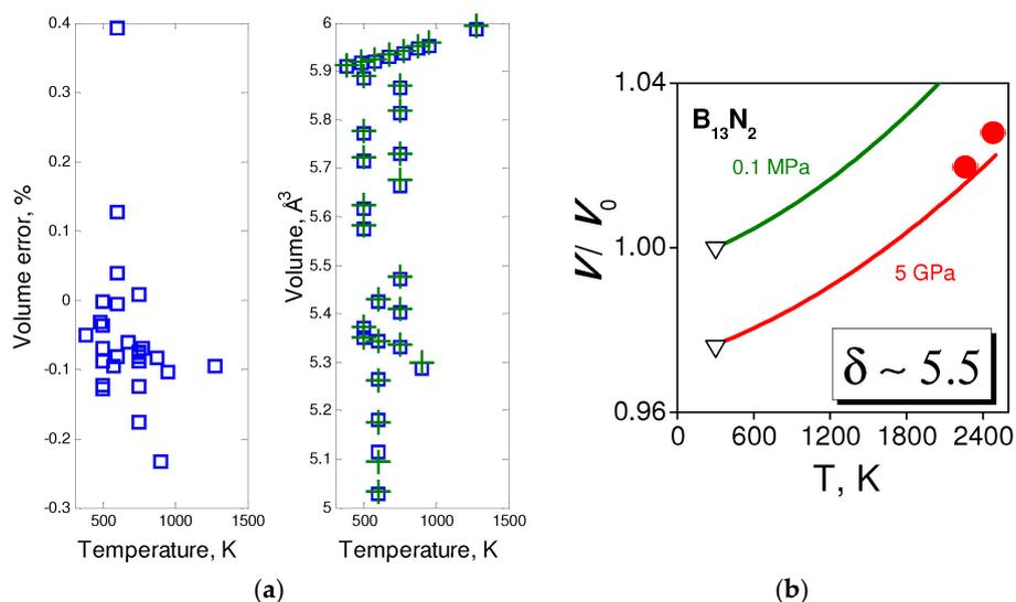
**Figure 6.**  $p$ - $V$ - $T$  equations of state: (a) cBN, experimental data from [60], adjusted to  $p$ - $V$ - $T$  EOS; and (b)  $B_{13}N_2$ , experimental data from [62], adjusted theoretical values for EOS parameters.
