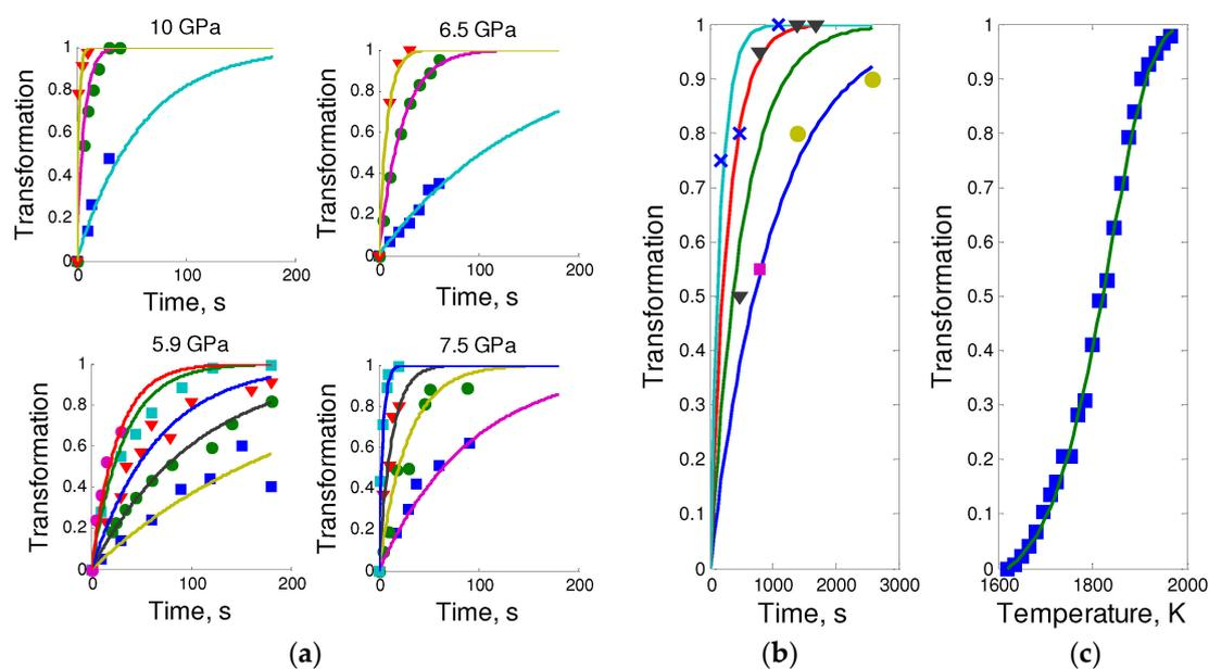
**Figure 8.** Kinetic curves for hBN-to-cBN transformation (all theoretical curves calculated using Equations (5) and (6)): (a) Top: isothermal kinetic data from [83] for pure pyrolytic hBN; bottom: isothermal kinetic data from [84] for hBN of technical grade; (b) isothermal kinetic data from [67] for pure hBN; and (c) non-isothermal kinetic data (linear heating, heating rate  $\beta = 10$  K/s) from our in situ observations for pure hBN obtained by thermally induced ordering of tBN.
