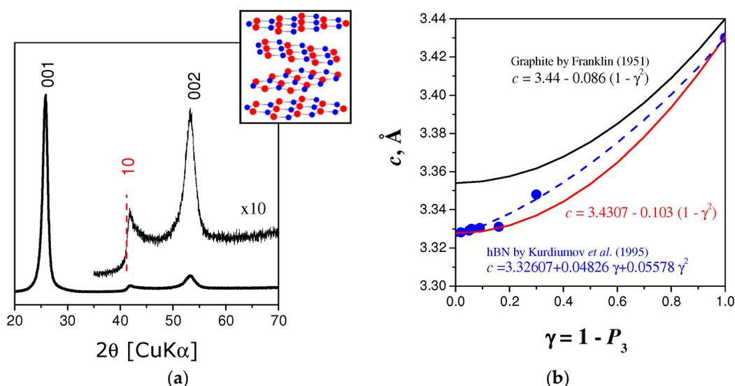
**Figure 2.** Crystal structure of turbostratic BN described in the framework of the random-layer lattice model: (a) Typical powder diffraction pattern with approximately symmetric  $00l$  reflections and strongly asymmetric two-dimensional  $hk$  reflections (with displaced maximum), *insert*: randomly displaced and rotated BN layers forming turbostratic structure; (b) Interlayer distance of turbostratic BN samples with different degree of turbostratic disorder.
