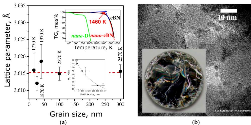
**Figure 4.** (a) Lattice parameters of nano-cBN as a function of grain size; oxidation stability (top inset) and hardness vs. grain size (bottom inset); (b) TEM image of nano-cBN grains and the view of the bulk sample recovered from HPHT (inset).
