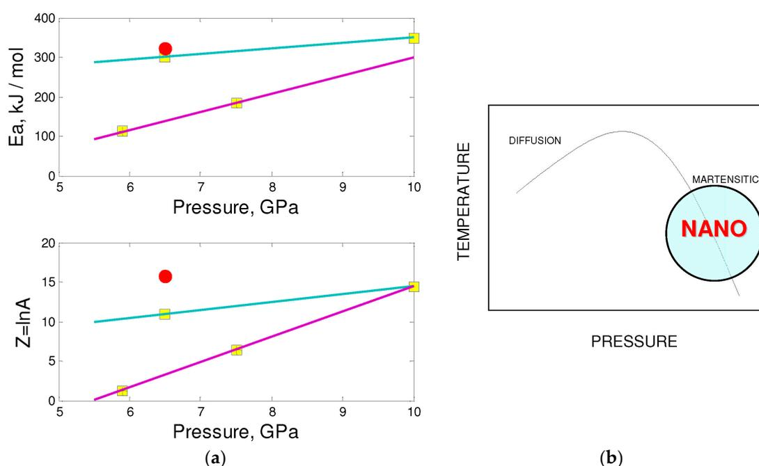
**Figure 9.** Kinetic parameters for hBN-to-cBN transformation: (a) Activation energy (top) and logarithm of pre-exponential factor (bottom) as function of pressure (open squares for pyrolytic hBN, crossed squares for hBN of technical grade, open circles for pure hBN obtained by thermally induced ordering of tBN); (b) Pressure-temperature diagram indicating the relative position of diffusive and displacive (martensitic) mechanisms. The latter favor the formation of nanostructures.
