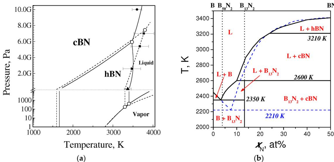
**Figure 7.** (a) Equilibrium phase  $P,T$ -diagram of boron nitride (solid lines—the refined diagram [69], dashed lines—diagram of 1988 [68]). Solid squares show Wentorf's data on hBN melting [66], solid circle is the melting point of cBN at 10 GPa [76], and solid triangle is hBN melting point at 50 MPa [74]; (b) Phase diagram of the B–BN system at 5 GPa [62]. Solid and dashed lines show the equilibrium and metastable phase diagrams respectively.
