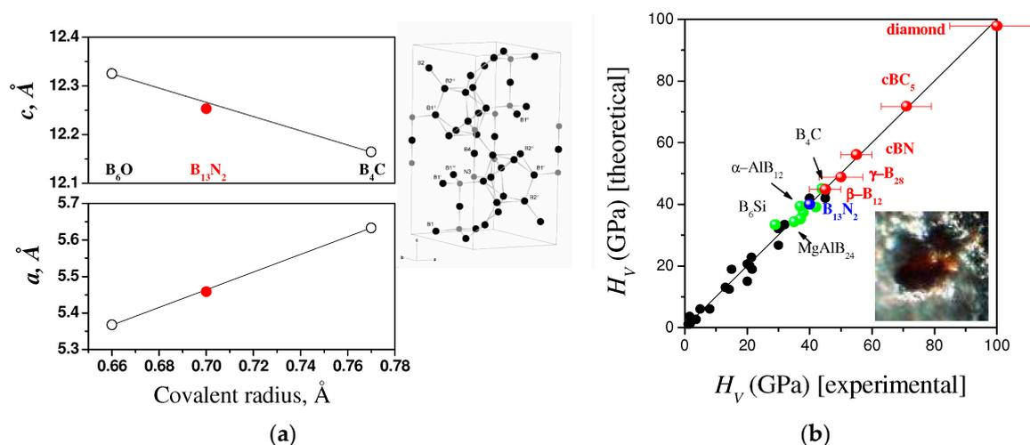
**Figure 3.** (a) Lattice parameters of boron subnitride  $B_{13}N_2$  as compared to other compounds with  $\alpha$ -B crystal structure; (b) Expected hardness of  $B_{13}N_2$  as compared to other superhard phases.
