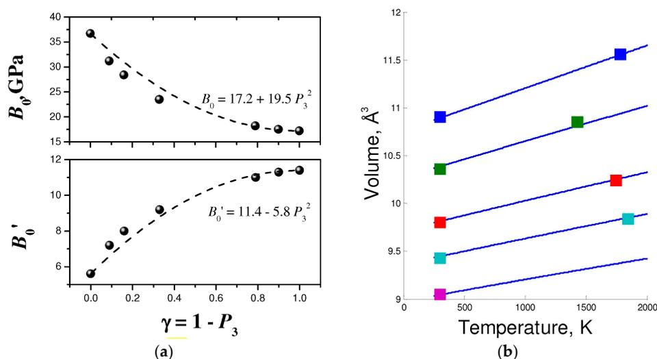
**Figure 5.** Equations of state of layered BN forms: (a) Bulk moduli and their pressure derivatives as a function of structural disorder along  $c$ -axis [58]; dashed lines show the model with only  $P_3^2$  term by analogy to lattice parameter dependence (Figure 2b); and (b) isobars (from top to bottom: 0.1 MPa, 2 GPa, 5.2 GPa, 8 GPa and 12 GPa) for hBN, experimental data from [59], adjusted to the  $p$ - $V$ - $T$  EOS.
