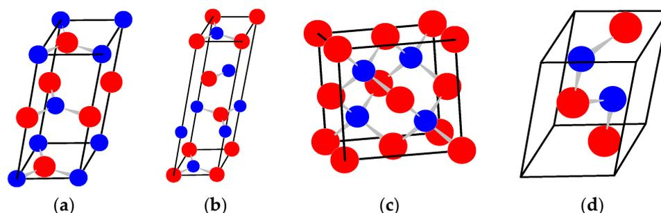
**Figure 1.** Crystal structures of BN polymorphs: (a,b) graphite-like hexagonal (hBN, 2H) and rhombohedral (rBN, 3R) low-density BN polytypes; and (c,d) cubic/sphalerite (cBN, 3C) and hexagonal/wurtzite (wBN, 2H) dense BN polytypes. The crystallographic axes are oriented in traditional way ( $\mathbf{u}_x \times \mathbf{u}_y \parallel \mathbf{u}_z$ ), and the coordinate origin (0; 0; 0) is in the front-left-bottom corner.
