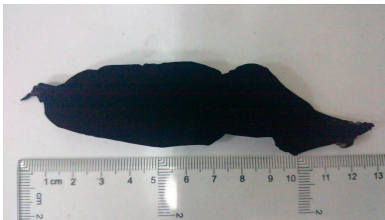
Figure S1. Optical image of as-grown CNT film. Size: 12 cm × 4 cm.
