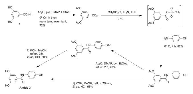
Scheme 3. Reagents, conditions and product yields obtained for the preparation of the amide selectophore 3 and its precursor intermediates.
