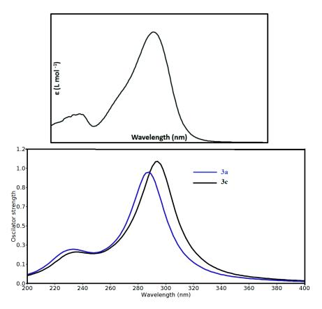
**Figure 5.** Experimental (**upper**) and calculated (**lower**) electronic spectra of the studied compounds using TD-DFT method.
