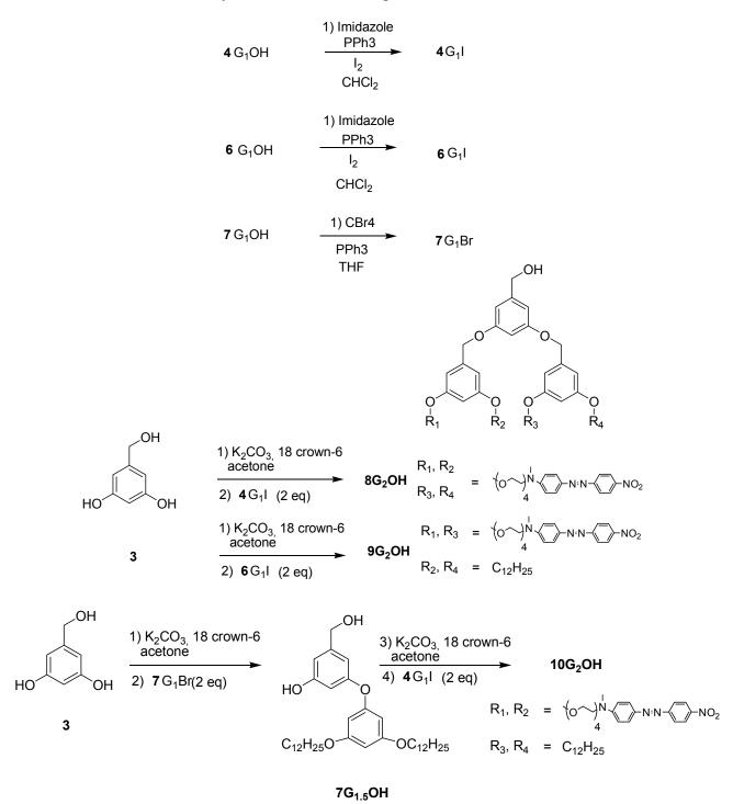
Scheme 2. Synthesis of the second generation dendritic molecules.
