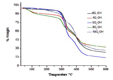
Figure 2. TGA of the obtained dendritic compounds.
