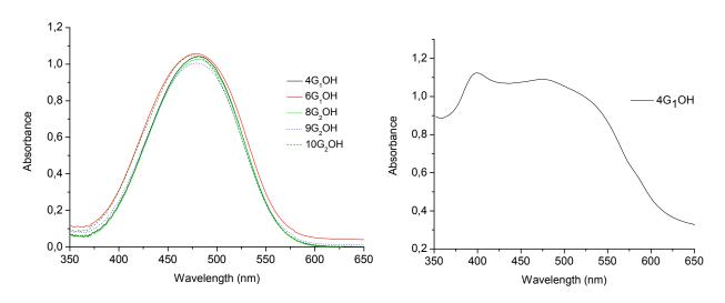
Figure 5. Absorption spectra of the obtained compounds: in solution (left) and in cast film (right).
