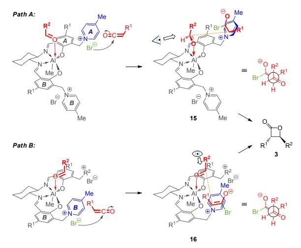
In *path B* the same aldehyde H atom would point away from the chiral salen backbone. To form the product with the observed absolute configuration again the *Re*-face of the aldehyde has to react and this would require the action of the other pyridinium moiety *B*.
