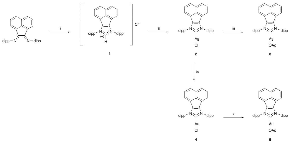
*Reagents and Conditions:* (i) MeOCH<sub>2</sub>Cl, 100 °C, 16 h; (ii) Ag<sub>2</sub>O, CH<sub>2</sub>Cl<sub>2</sub>/THF, 25 °C, 16 h; (iii) AgOAc, CH<sub>2</sub>Cl<sub>2</sub>, 25 °C, 12 h; (iv) (tht)AuCl, CH<sub>2</sub>Cl<sub>2</sub>, 25 °C, 12 h; (v) AgOAc, CH<sub>2</sub>Cl<sub>2</sub>, 25 °C, 12 h.
