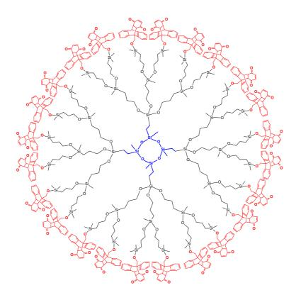
Versatile dendrimers of a siloxane core [38] and bicyclo-groups on the periphery having 96 endgroups were prepared. The structural information of the Diels-Alder product on the dendritic periphery is obtained from the hyperfine structure of the products' NMR spectra. The purity of the product is determined by size exclusion chromatography [39].
