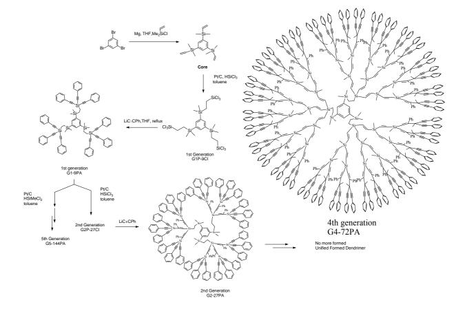
The ethylnyl groups of each generation is reacted with  $Co_2(CO)_8$ , which is reported by Kim *et al.* to give hexacarbonyl tetrahedron structures having up to 32 ethylnyl groups on the periphery [19]. The 2nd generation of ethylnyl silane and its hexacarbonyl tetrahedron structures were confirmed by MALDI TOF mass spectroscopy (Scheme 6).
