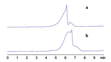
Determination of the molecular weight of ASP-I and APS-II by HPLC-GPC run in isocratic mode. Mobile phase: 100% water; the column and optical unit of RID were set at 30°C and 35°C, respectively; flow rate, 1.0 mL/min; injection volume, 10 mL; (a) APS-I, retention time 6.162 min; (b) APS-II, retention time 6.397 min.
