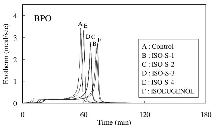
**Figure 2.** Time-conversion curves for the polymerization of MMA initiated by thermal decomposition of BPO in the presence of 0.01 mol% additives. Curves were obtained from findings shown in Figure 1.
