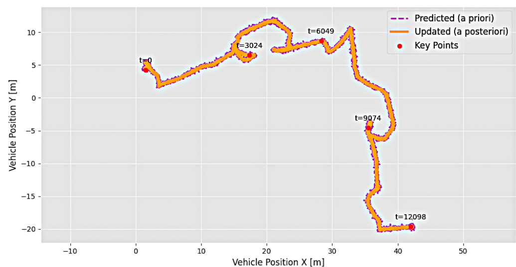
Figure 6. Position uncertainty reduction after multimodal fusion. The Kalman Filter is used only as a reference estimator for comparison.
