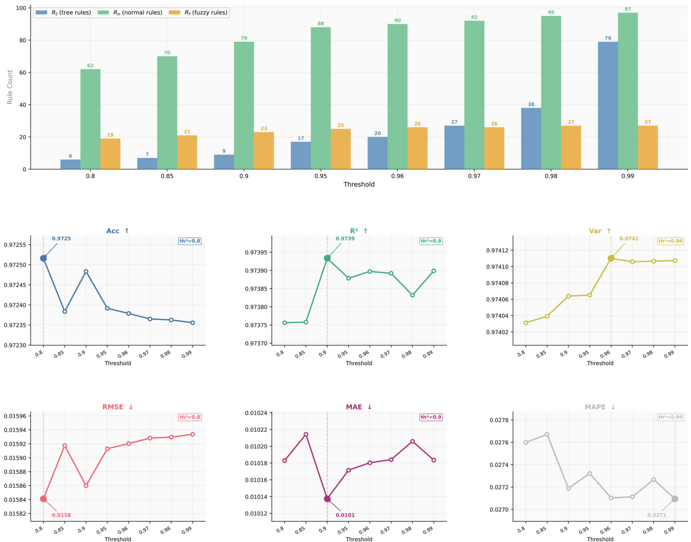
Figure 8. Sensitivity of forecasting performance and Tucker ranks to the PCA threshold for Tucker rank selection.
