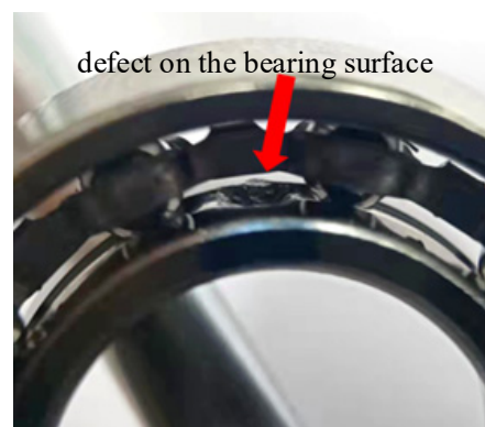
Figure 14. Realistic image of the defect on the bearing surface.
