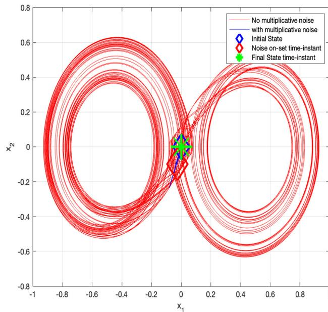
**Figure 3.**  $x_1$  vs.  $x_2$  : Chaos stabilization using multiplicative noise, the original  $\sigma = 0$  jumps to  $\sigma = 3$  at  $t = 500$  s.
