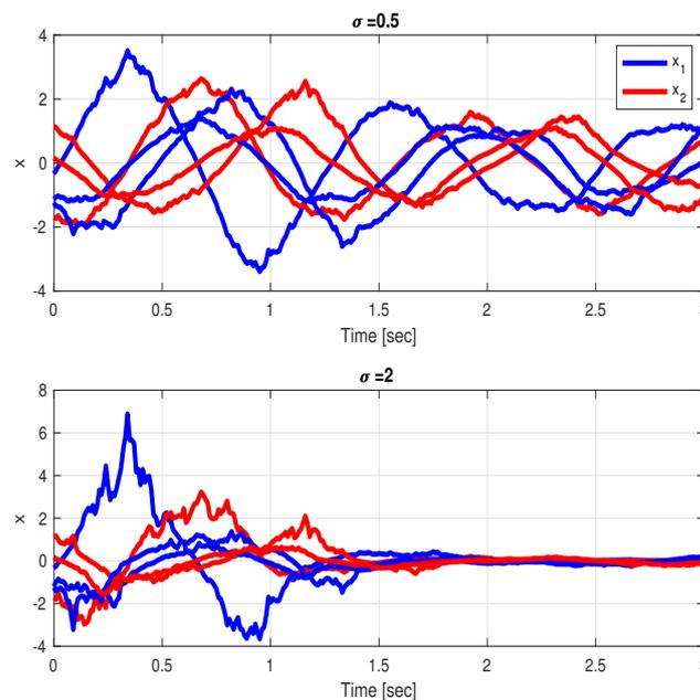
**Figure 2.** Second-order system subject to state-multiplicative noises of different intensities, (top) For  $\sigma = 0.5$ ,  $\bar{\lambda}(A + A^T) > \sigma^2$ , SAR not attained, (bottom) For  $\sigma = 2$ ,  $\bar{\lambda}(A + A^T) < \sigma^2$ , SAR attained.
