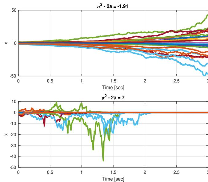
**Figure 1.** A scalar system that is unstable without state-multiplicative noise, (**top**)  $\sigma^2 < 2a$  SAR not attained, (**bottom**)  $\sigma^2 > 2a$  SAR attained.
