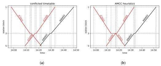
**Figure 3.** A possible solution of the conflict on line No. 216. (a) The conflicted diagram. All the three trains would meet in block 4 as it can be seen from the intersecting train paths. (b) The solution; FCFS, FLFS, and AMCC give the same outcome with a maximum seconday delay of 4 min.
