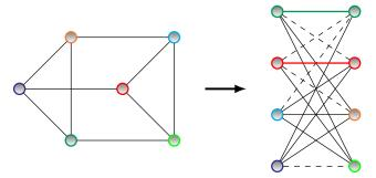
**Figure 6.** Embedding of a simple, six-qubit problem. (**Left**) graph of the original problem. (**Right**) problem embedded into a unit cell of Chimera. Here, different colors correspond to different logical variables. Apparently, the original problem does not map directly onto Chimera as it contains cycles of length 3. Therefore, two chains have to be introduced. Couplings corresponding to inner-chain penalties are marked with the same color as the variable to which they correspond.
