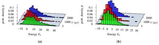
**Figure 5.** Distribution of the energies corresponding to the states (solutions), which are sampled by the D-Wave 2000Q quantum annealer of 48 logical quantum bits instance of line No. 216. In particular, 1000 samples were taken for each annealing time, and the strength of embedding was set to css = 2.0. This device is still very noisy and prone to errors, so the sample contains excited states. (a) QUBO param.:  $p_{pair} = 2.7$ ,  $p_{sum} = 2.2$ . (b)  $p_{pair} = p_{sum} = 1.75$ .
