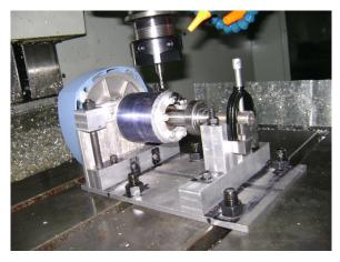
Figure 4. Rotor bar drilling to create the damage levels.
