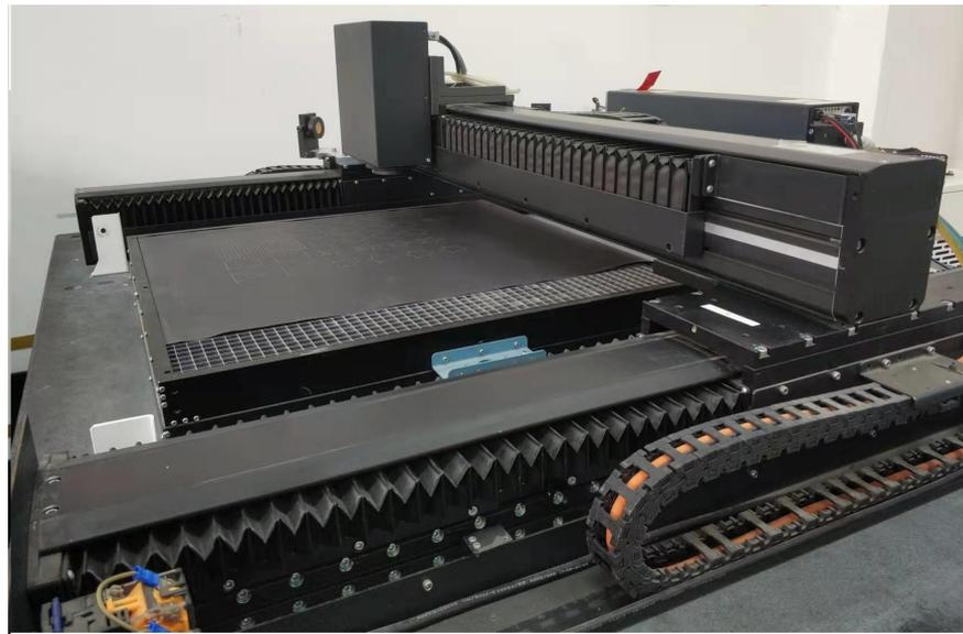
Figure 2. Dual-drive gantry stage.
