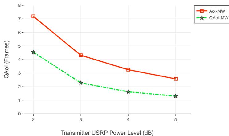
Figure 12. Evaluation of QAoI ( $J_Q$ ) for varying power levels of transmitter USRP, 25 frames length query period.
