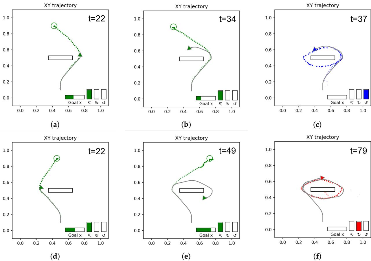
**Figure 13.** Anticipated goal and trajectories as the network observes the cyclic trajectories. The colored dots represent the anticipated trajectory, while the solid gray line is the observed trajectory. The time step is shown in the top right. (a–c) Agent following the counter-clockwise cyclic goal trajectory, (d–f) agent following the clockwise cyclic goal trajectory.
