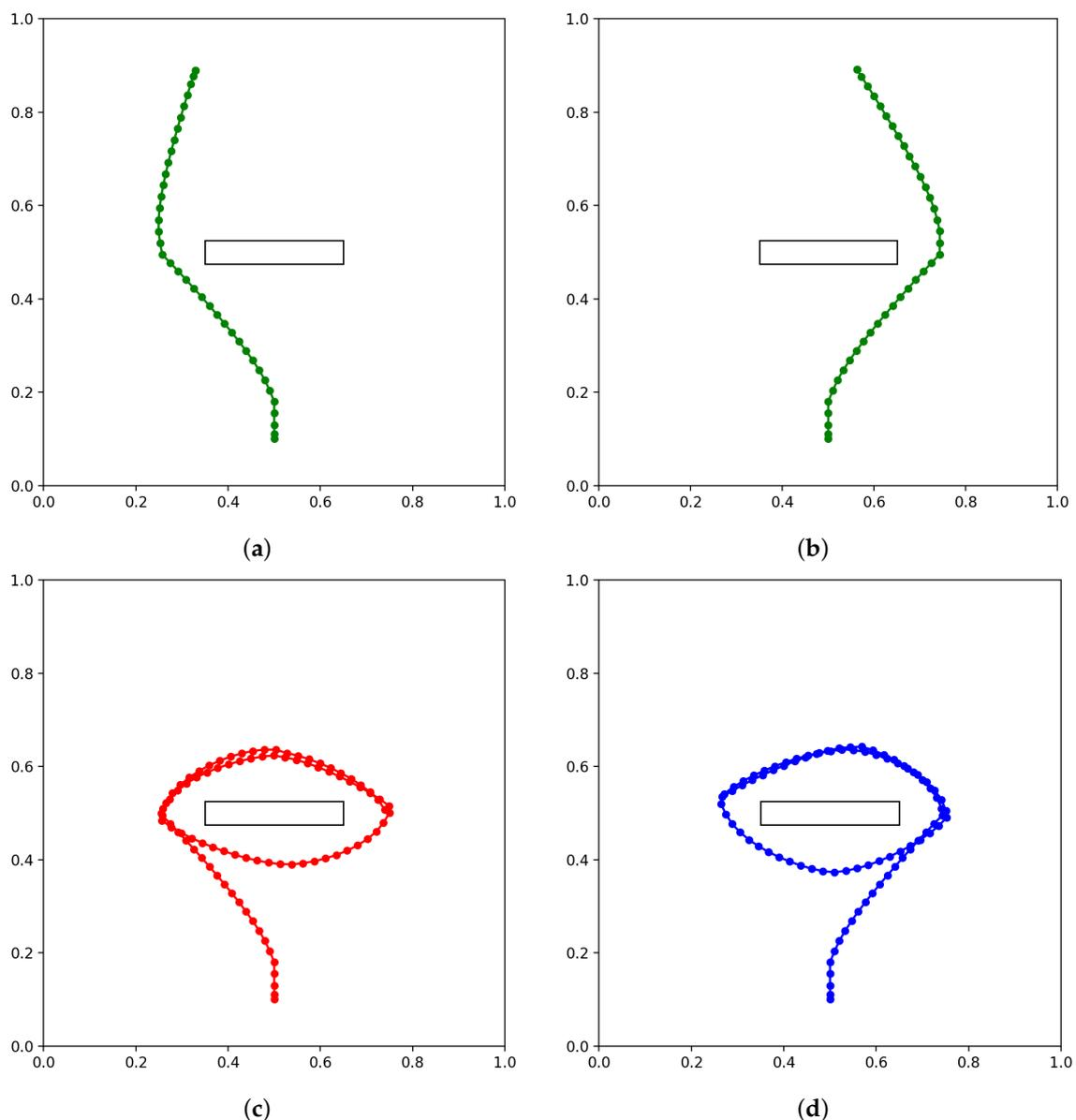
**Figure 11.** Test trajectories used for goal inference, color coded by the type of goal. These trajectories represent agent actions for (a) reaching goal located on the left, (b) reaching goal located on the right, (c) clockwise cycling, and (d) counter-clockwise cycling. The reaching trajectories and the cycling trajectories are 40 and 90 steps long, respectively.
