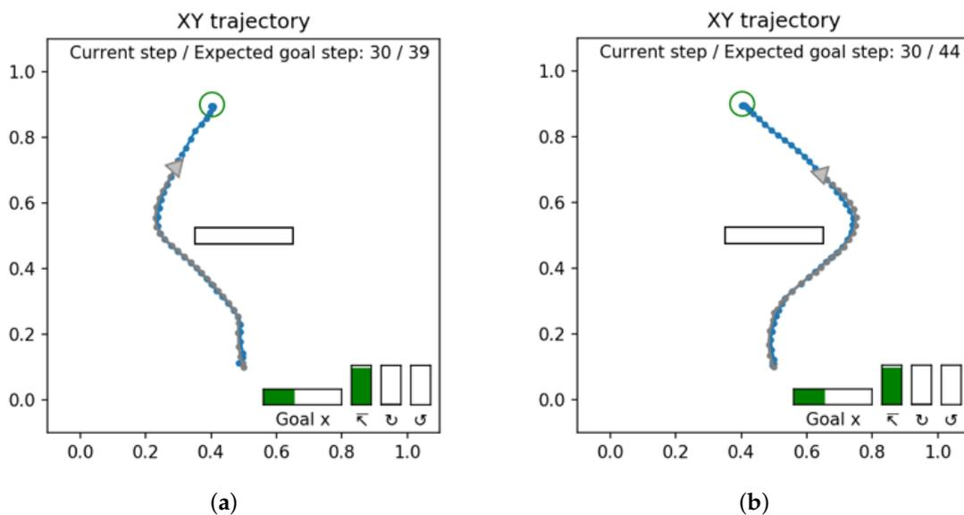
**Figure 15.** Examples of ill-posed goal-directed planning. (a) Generation of a short path reaching the goal (39 time steps) and (b) an alternative long path to the same goal (44 time steps).
