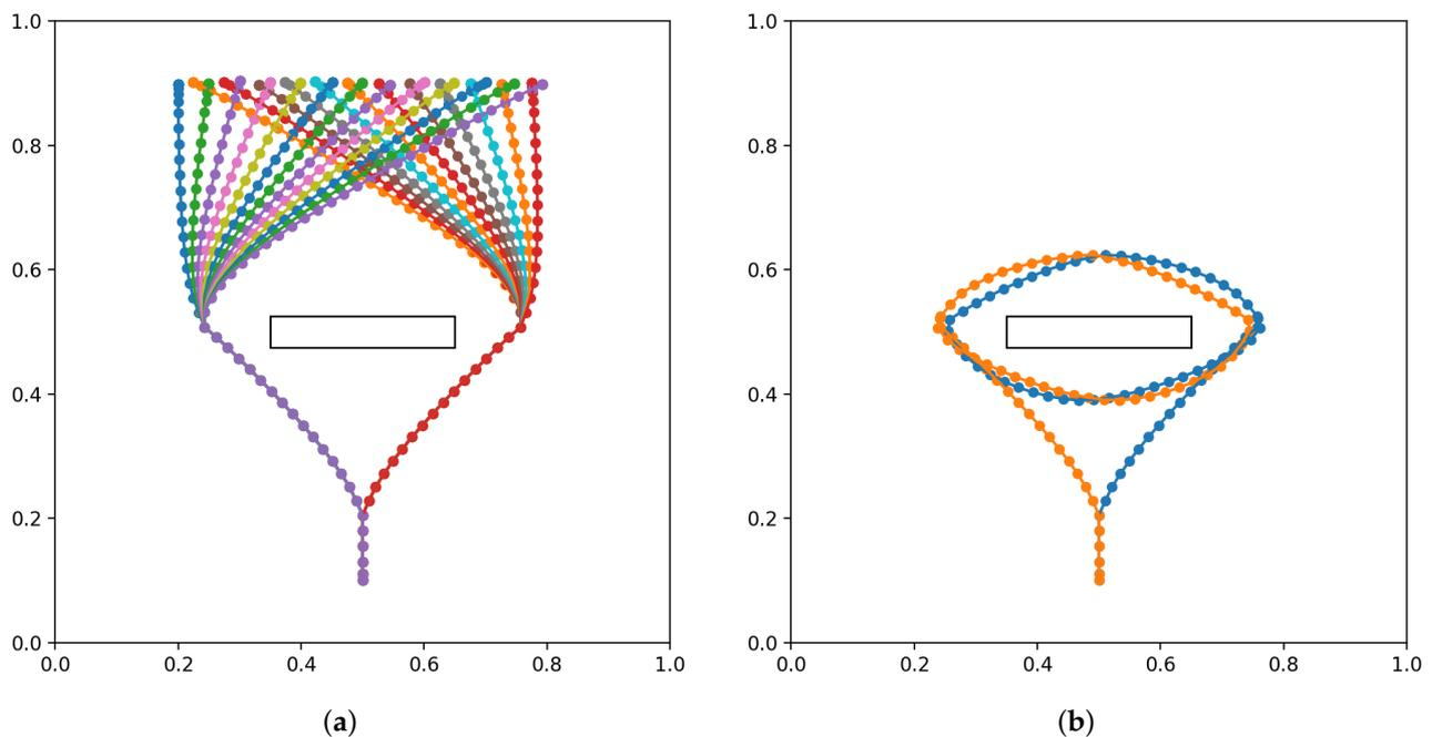
**Figure 9.** Teaching trajectories used for Experiment 1B, with both goal-reaching and cycling goals. (a) 25 reaching trajectories, with both short and long paths (b) 2 cycling trajectories, in the clockwise and counter-clockwise directions
