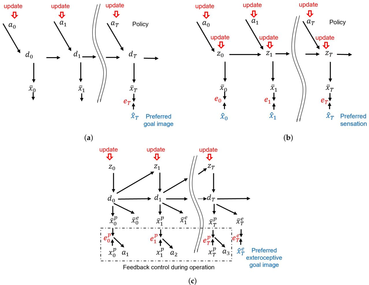
**Figure 1.** Prior models for generating goal-directed behaviors. (a) Forward model using latent variables, (b) active inference model using probabilistic latent variables, and (c) GLearn as an extension of active inference.
