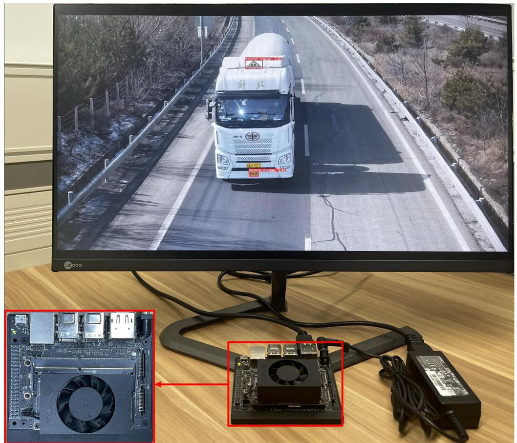
**Figure 5.** The actual deployment of HMD-Net on Jetson Xavier NX.
