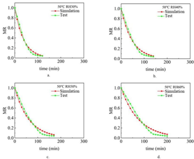
**Figure 6.** The simulated and experimental values of the change of the sludge moisture ratio MR with the drying time  $t$  when the air temperature is  $50\text{ }^{\circ}\text{C}$  after considering the shrinkage effect and the crack phenomenon in the sludge drying process: (a) RH 30%, (b) RH 40%, (c) RH 50%, (d) RH 60%.
