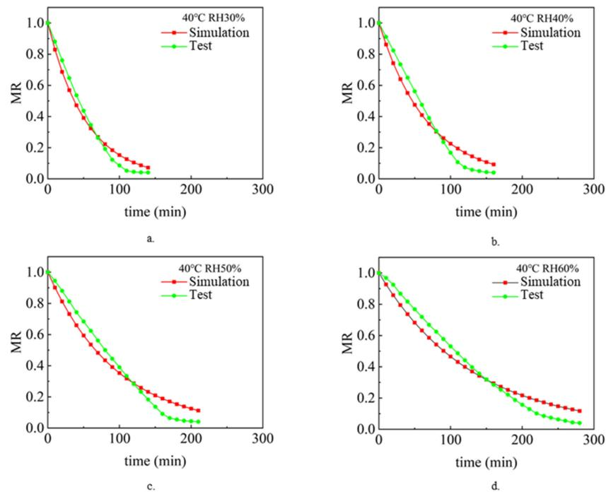
**Figure 5.** The simulated and experimental values of the change of the sludge moisture ratio MR with the drying time  $t$  when the air temperature is  $40\text{ }^{\circ}\text{C}$  after considering the shrinkage effect and the crack phenomenon during the sludge drying process: (a) RH 30%, (b) RH 40%, (c) RH 50%, (d) RH 60%.
