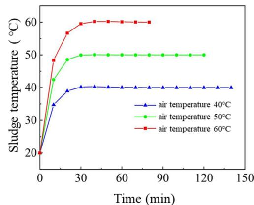
**Figure 8.** The average temperature rise curve inside the sludge at different air temperatures under the condition of 30% relative air humidity.
