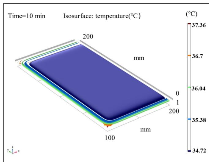
**Figure 9.** Isothermal surface distribution cloud map of average sludge temperature at 10 min.
