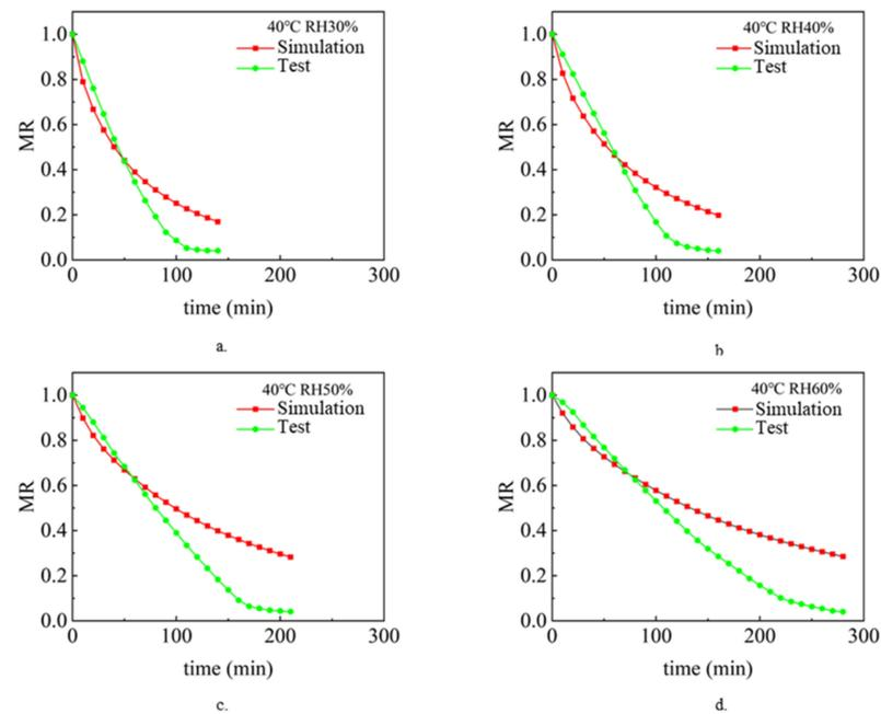
**Figure 2.** The simulated and experimental values of the change of the sludge moisture ratio MR with the drying time  $t$  when the air temperature is 40 °C: (a) RH 30%, (b) RH 40%, (c) RH 50%, (d) RH 60%.
