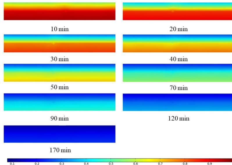
**Figure 13.** MR distribution cloud map of sludge moisture ratio in a section of the sludge center at different times under the conditions of air temperature 50 °C and air relative humidity 50%.
