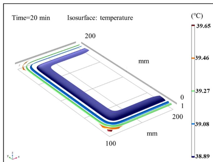
**Figure 10.** Isothermal surface distribution cloud map of average sludge temperature at 20 min.
