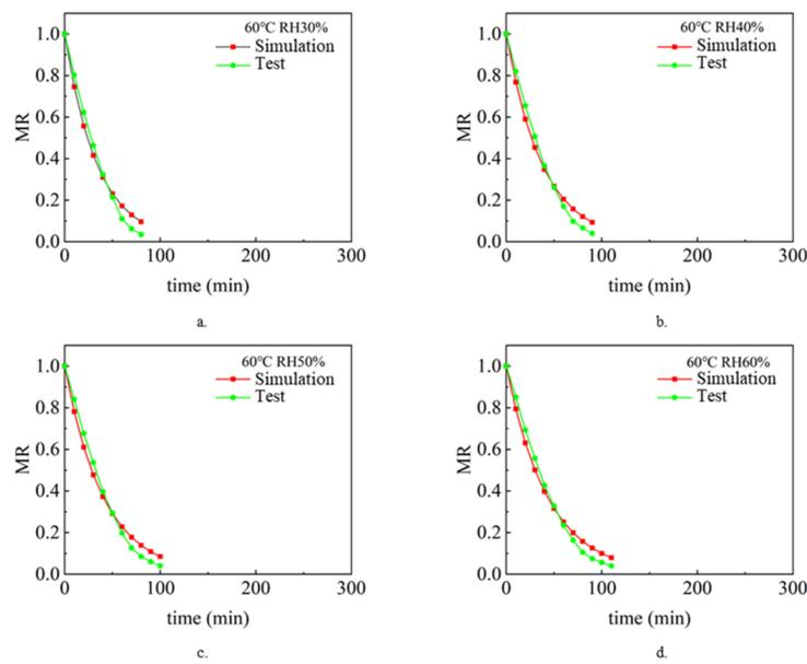
**Figure 7.** The simulated and experimental values of the change of the sludge moisture ratio MR with the drying time t when the air temperature is 60 °C after considering the shrinkage and cracks during the sludge drying process: (a) RH 30%, (b) RH 40%, (c) RH 50%, (d) RH 60%.
