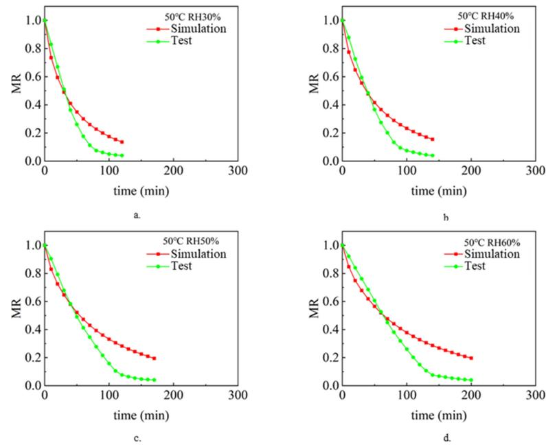
**Figure 3.** Changes of sludge moisture ratio MR with drying time  $t$  when the air temperature is 50 °C: (a) RH 30%, (b) RH 40%, (c) RH 50%, (d) RH 60%.
