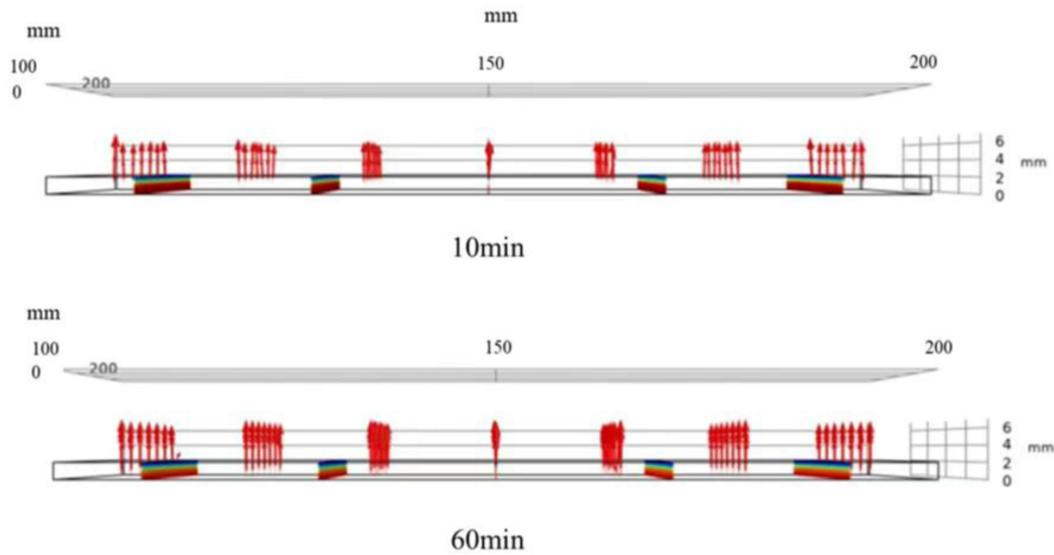
**Figure 12.** Under the condition of an air temperature of 50 °C and relative air humidity of 50%, the diffusion direction of water inside the sludge at different temperatures of 10 min and 60 min.
