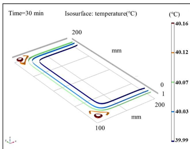
**Figure 11.** Cloud map of the isothermal surface distribution of average sludge temperature at 30 min.
