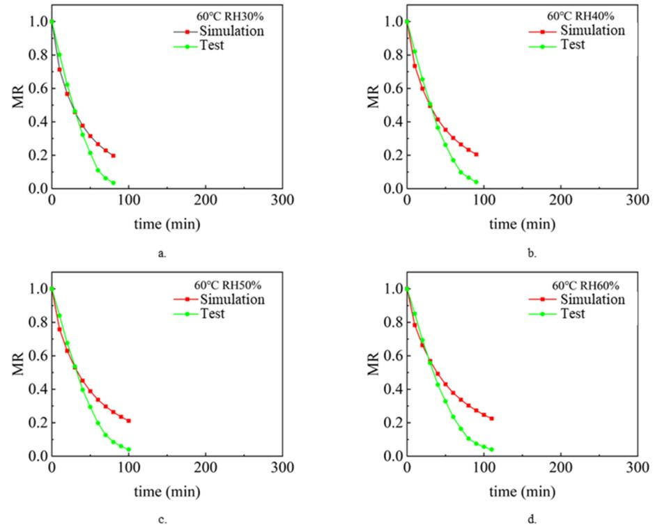
**Figure 4.** Variation of sludge moisture ratio MR with drying time  $t$  when the air temperature is 60 °C: (a) RH 30%, (b) RH 40%, (c) RH 50%, (d) RH 60%.
