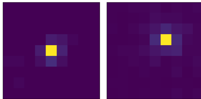
Figure 3. Samples of signal amplitudes for hits on (0, 0) and (20, 20) mm, respectively, where brighter color indicates a larger increase in amplitude.
