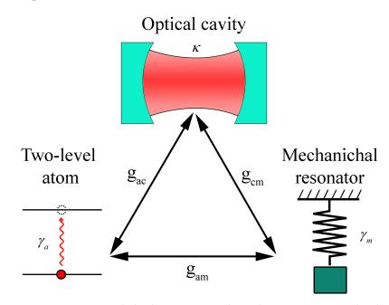
**Figure 1.** A tripartite hybrid system: A single-mode e.m. cavity, a two-level atom and a mechanical resonator are coupled to each other via the coupling strengths  $g_{ac}$ ,  $g_{cm}$ , and  $g_{am}$ .
