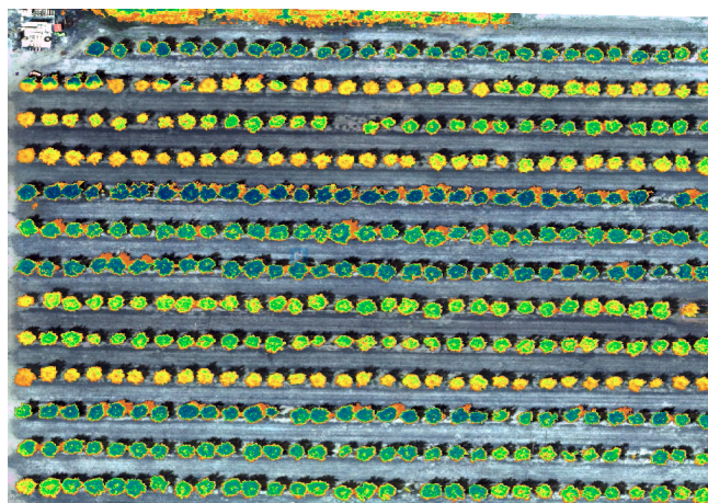
Figure 7. Normalized difference vegetation index (NDVI) mapping of pomegranate trees.
