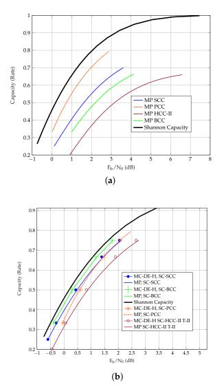
**Figure 6.** Comparison of TC ensembles in terms of the AWGN channel Thresholds. (a)  $E_b/N_0$  vs. Rate of uncoupled TCs. (b)  $E_b/N_0$  vs. Rate of SC-TCs with m = 1.
