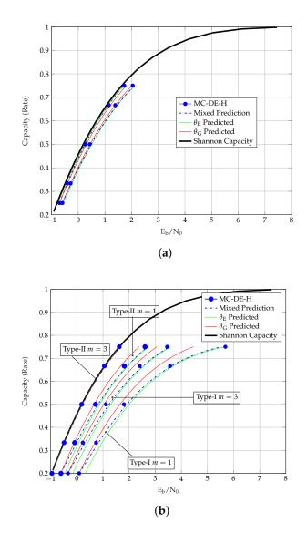
**Figure 4.** Thresholds of SC-SCCs and SC-HCCs over the AWGN channel. (a)  $E_b/N_0$  vs Rate of SC-SCCs with m = 1 and m = 3. (b)  $E_b/N_0$  vs Rate of type 1 and type 2 SC-HCCs-II with m = 1 and m = 3.
