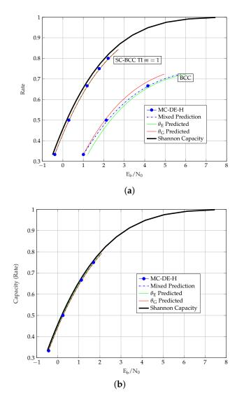
**Figure 5.** Thresholds of BCCs over the AWGN channel. (a)  $E_b/N_0$  vs. Rate of BCCs and SC-BCCs with m = 1. (b)  $E_b/N_0$  vs. Rate of SC-BCCs with m = 3.
