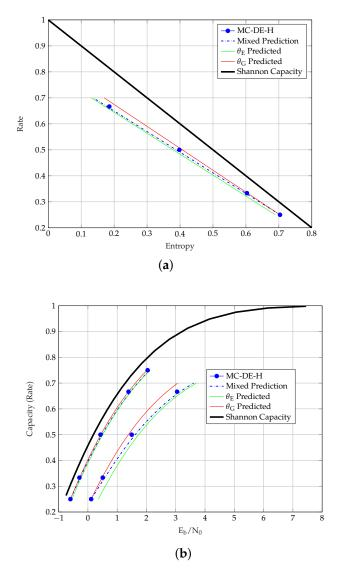
**Figure 2.** AWGN channel thresholds of uncoupled and coupled SCCs. (a) SCC Entropy vs. Capacity. (b) SCC and m = 1 SC-SCC  $E_b/N_0$  vs. Capacity.
