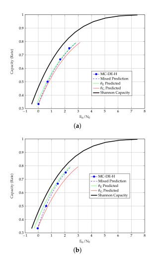
**Figure 3.** Thresholds of PCCs over the AWGN channel. (a)  $E_b/N_0$  vs. Rate of PCC. (b)  $E_b/N_0$  vs. Rate of m = 1 SC-PCC.
