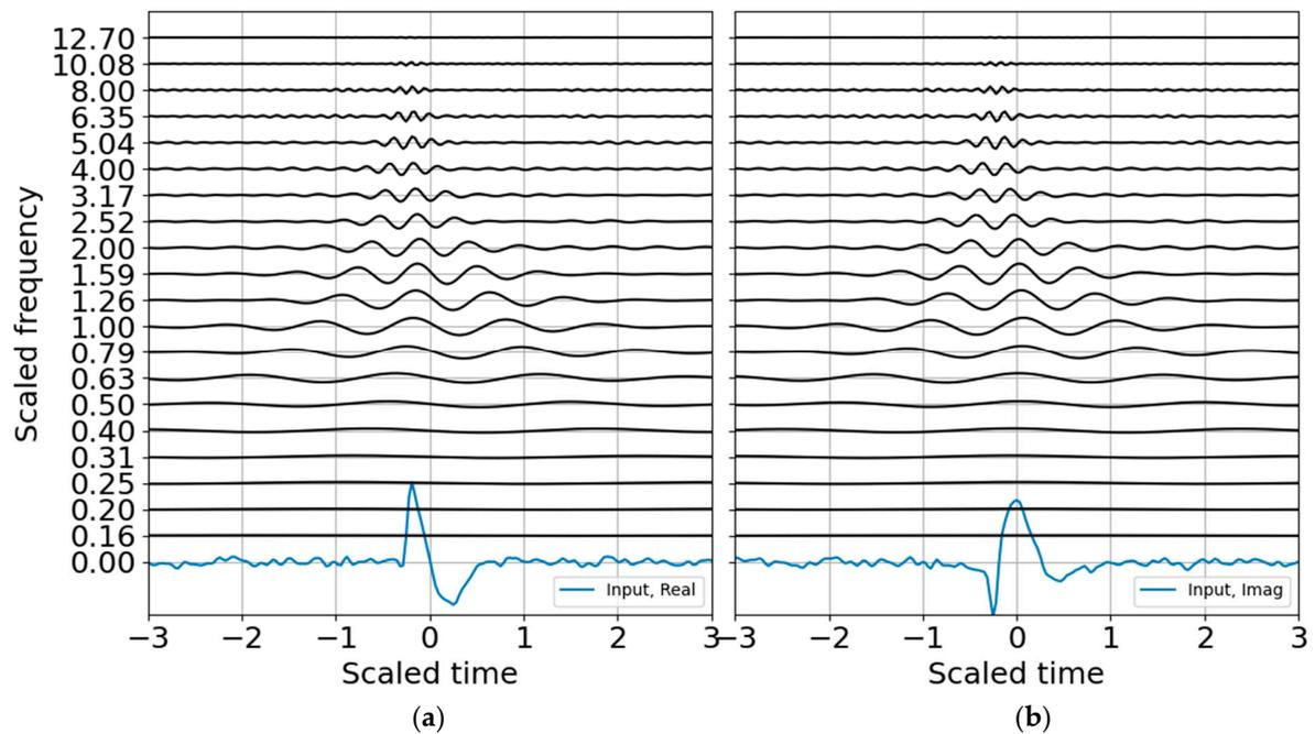
**Figure 4.** Wavelet decomposition with 1/3 octave bands, with CWT amplitudes scaled by the reconstruction coefficients. (a) Real part; (b) imaginary part. As with Figure 1, the input waveform is displayed at the zero frequency.
