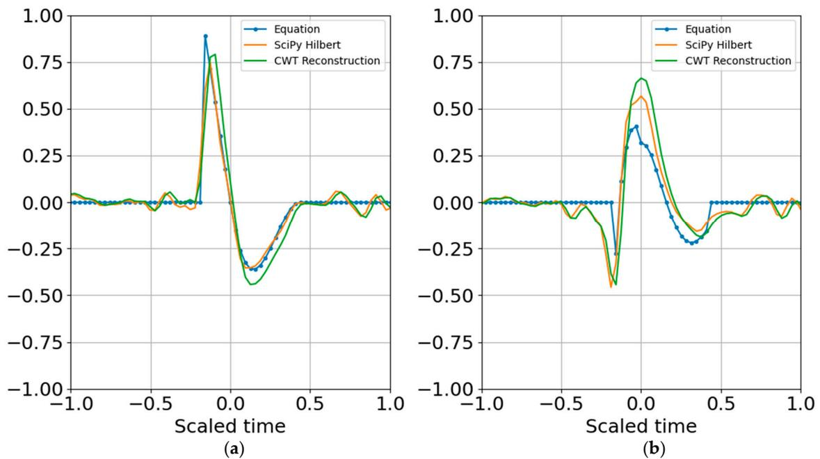
**Figure 2.** Wavelet reconstruction with binary bands. (a) Real part; (b) imaginary part. The Equation waveform has no noise and is not filtered, whereas Hilbert has Gaussian noise and has been anti-aliased filtered.
