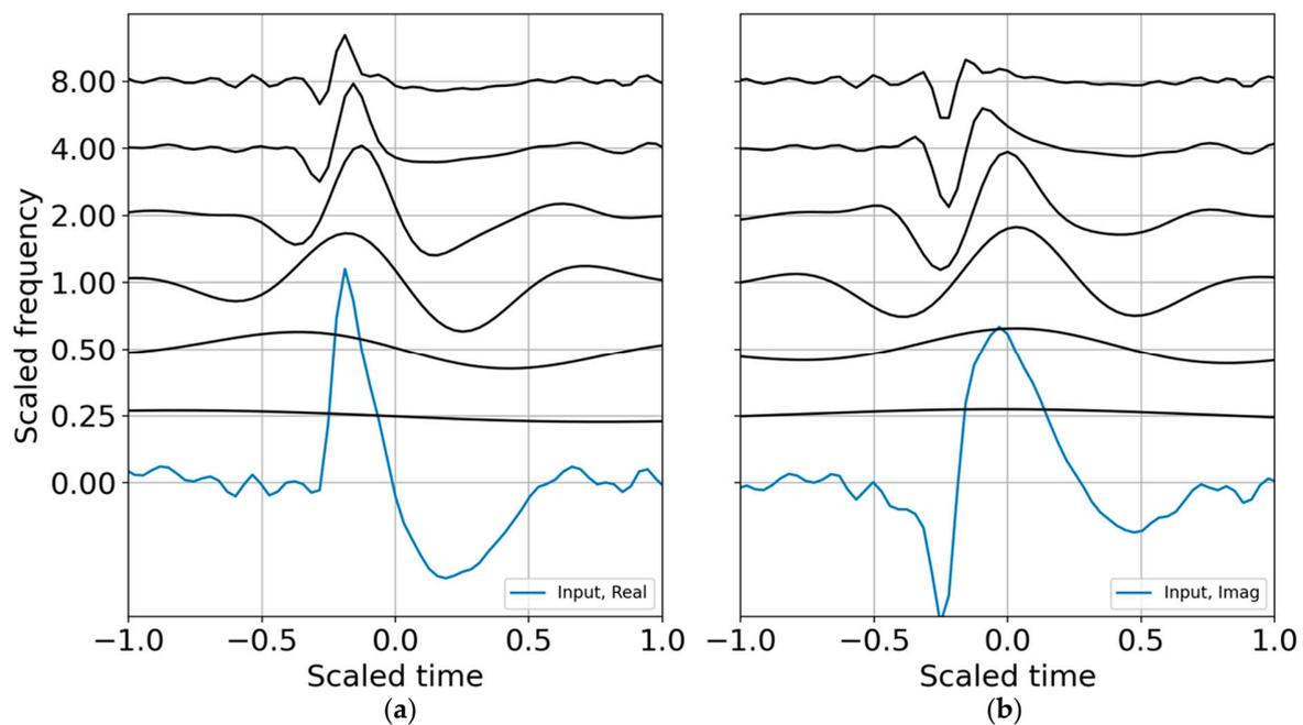
**Figure 1.** Analytic signal from mathematical equation, computation with SciPy Hilbert, and the continuous wavelet transfer (CWT) reconstruction. (a) Real part; (b) imaginary part. The wavelets were evaluated in binary bands ( $N = 1$ ) and constructed around the target frequency of 6.3 Hz, which scales frequency and time. The real input waveform and its computed Hilbert transform are displayed in blue at the zero frequency.
