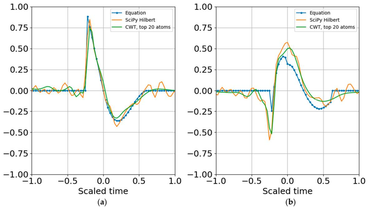
**Figure 11.** (a) Real part and (b) imaginary part of the original and reconstructed waveform. Increasing the noise amplitude so that its variance is the same as the signal variance still permitted reconstruction from the superposition of the largest atoms per band.
