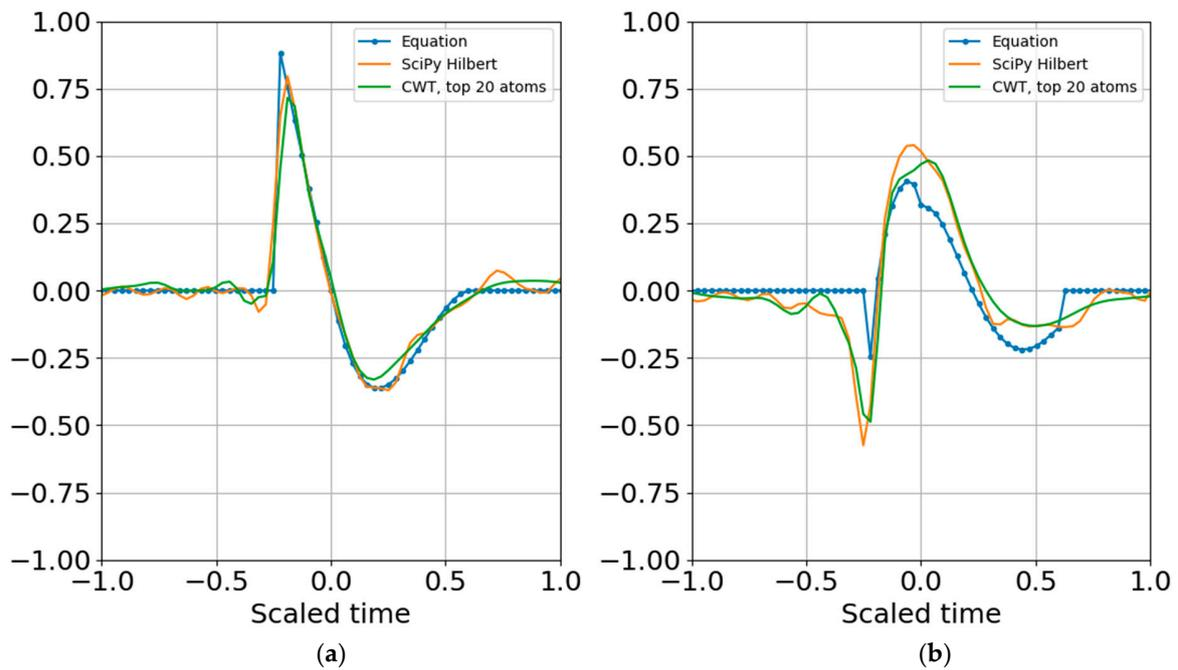
**Figure 9.** Superposition of largest SNR entropy coefficients per band using all twenty 1/3 octave bands. (a) Real part; (b) imaginary part. The noise standard deviation is one bit below the signal’s. Dimensionality is reduced to the number of coefficients and their corresponding time shifts.
