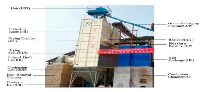
Figure 1. Picture of the industrial drying system.
