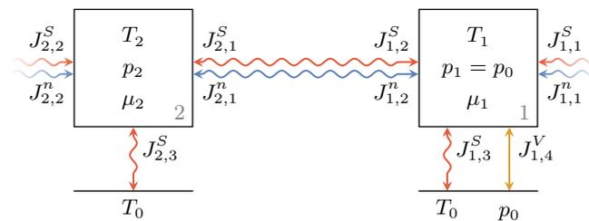
**Figure 2.** Endoreversible model of pipe segment (Reservoir 2) and hydraulic fluid tank (Reservoir 1) with combined particle and entropy fluxes between them and towards further pipe segments. Additionally, both reservoirs have irreversible heat transfers to the environment (line below), and the fluid tank is connected to the environment via a reversible volume flux.
