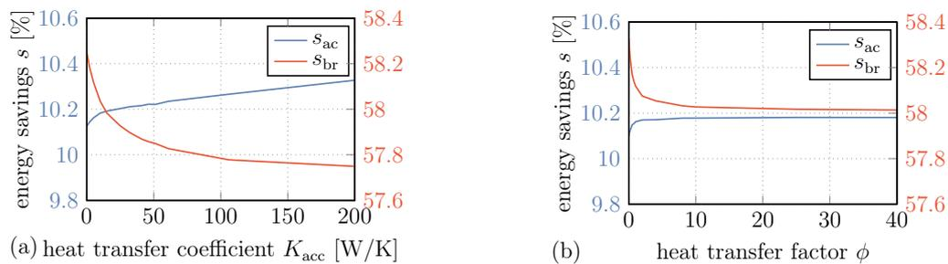
**Figure 12.** Energy savings both accelerating and decelerating the vehicle over heat transfer coefficient within the accumulator (a) and heat transfer factor (b). The latter scales the heat transfers of the pipes segments, the hydraulic fluid within the bladder accumulator and the hydraulic fluid tank to the environment.
