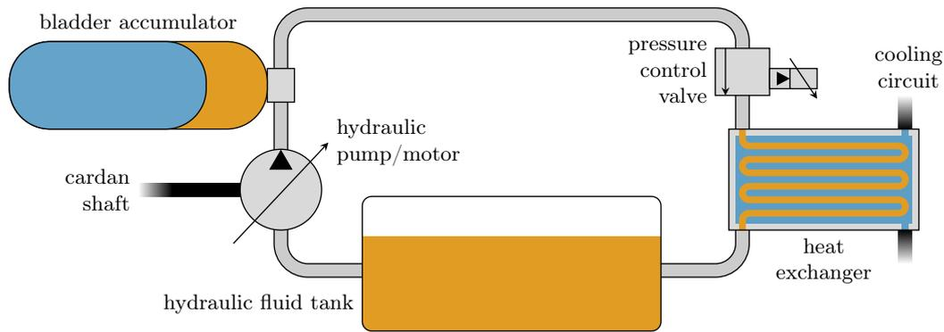
**Figure 1.** Scheme of the hydraulic recuperation system.
