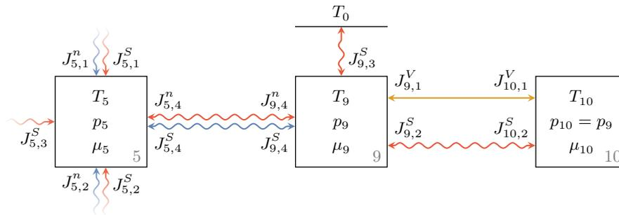
**Figure 5.** Endoreversible model of the bladder accumulator with adjacent pipe segment. Reservoirs 9 and 10 represent the hydraulic fluid and the gas within the bladder accumulator, respectively, which are connected via an irreversible heat transfer and a reversible volume flux. Further, there is an irreversible heat transfer from the hydraulic fluid to the environment.
