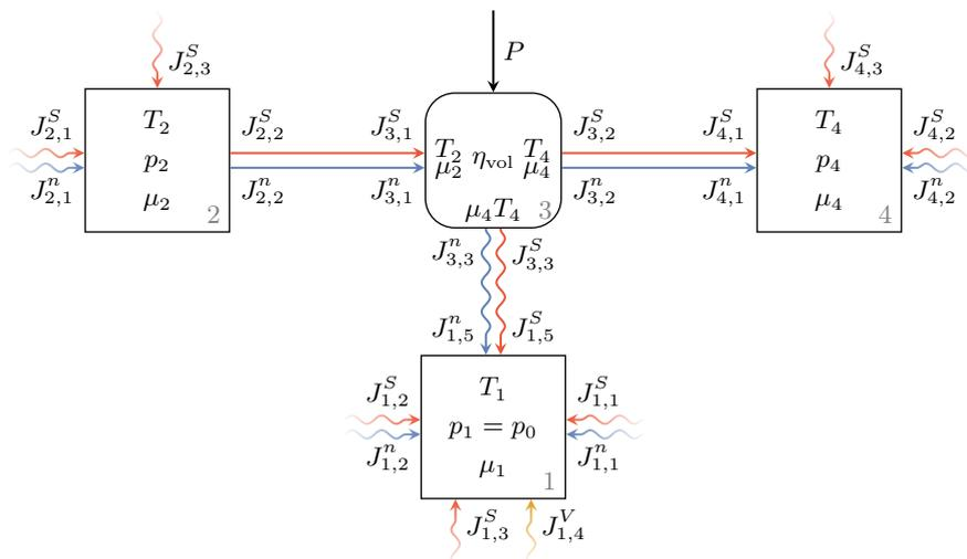
**Figure 3.** Endoreversible model of the hydraulic unit as a dissipative engine with given efficiency (Engine 3) and unspecified power input as well as hydraulic fluid tank and adjacent pipe segments (Reservoirs 1, 2 and 4, respectively). The flow directions are drawn according to the flow directions of the hydraulic unit operating in pump mode.
