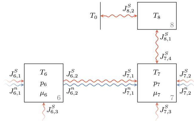
**Figure 6.** Endoreversible model of the pressure control valve represented by an irreversible combined particle and entropy flux between two pipe segments (Reservoirs 6 and 7). The valve housing (Reservoir 8) is connected to Reservoir 7 and the environment via irreversible heat transfers.
