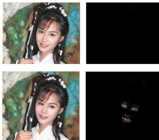
Figure 5. Samples of the original and tampered images and the error level analysis results.
