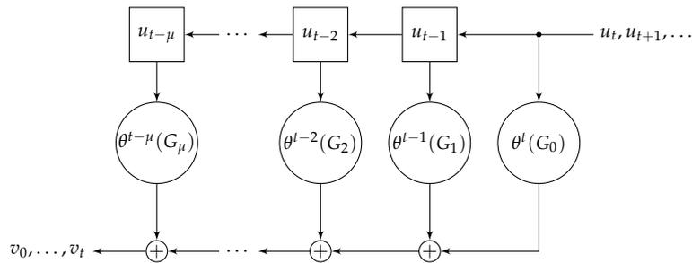
Figure 1. Encoder of a skew convolutional code.
