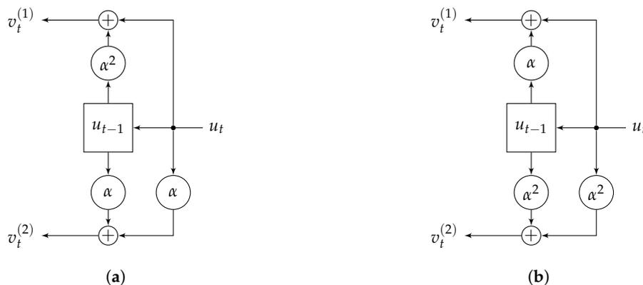
**Figure 2.** Encoder of the skew code  $\widehat{C}$  from Example 2: (a) for even  $t$ , (b) for odd  $t$ .
