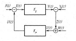
**Figure 1.** This is a figure from [1]. Here,  $K_0$  denotes the operator object which transform the input function X(t) to the output function Y(t) which should be compared with the given function  $Y_0$  (the program function). The "defect" signal *Z* together with a measurement "noise" *N* forms the input of a regulator given by an operator  $K_r$ . The resulting control signal *U* with an external perturbation *P* goes back to the input of the object operator  $K_0$ .
