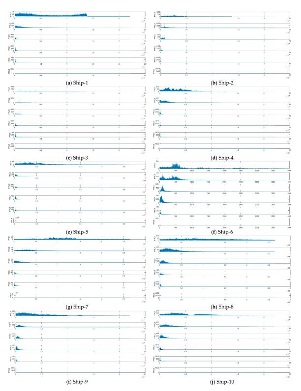
Figure 7. Spectrum of results of ITD for ten types of ship-radiated noise signals.
