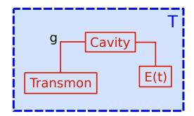
**Figure 1.** Sketch of the quantum engine with a transmon qubit as working substance interacting with an externally pumped (E(t)) transmission line (cavity). Both systems are embedded in the same cryogenic environment, which plays the role of a standard thermal bath of temperature *T*. Such a setup gives a dynamics of a working substance in the presence of a controllable *non-thermal* environment.
