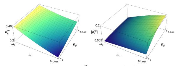
**Figure A1.** Stationary state's elements  $\rho_T^{ee}$  and  $|\rho_T^{eg}|$  for different values of  $(\omega_T, E_d)$ . Important amounts of population and quantum coherence changes can be reached during the engine operation.
