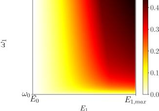
**Figure 4.** Efficiency  $\eta$  as a function of the upper values  $(\omega_1, E_1)$  for the cycle depicted in Figure 2. The observed highest efficiency of about 47% was attained when  $(\omega_1, E_1) = (\omega_{1,\max}, E_{1,\max})$ , with  $\omega_{1,\max}/2\pi = 1000$  MHz and  $E_{1,\max}/2\pi\hbar = 2$  MHz.
