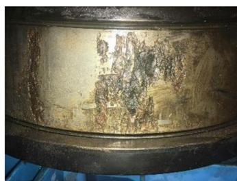
Figure 17. Peeling of the inner ring.
