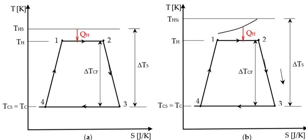
**Figure 3.** Representation of the associated cycle to the Chambadal engine in T-S diagram: (a) source of constant temperature; (b) source of finite heat capacity.
