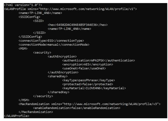
Figure 5. WiFi profile file created when the microSD is burnt.
