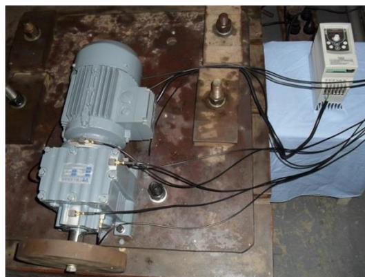
**Figure 1.** An experimental rig of simulating gear faults.
