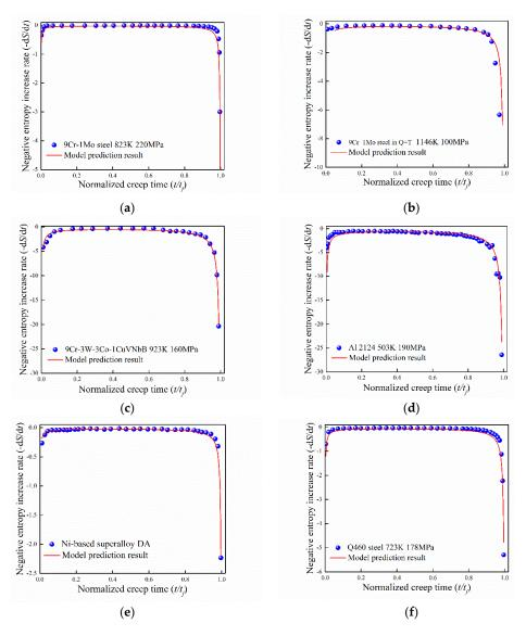
**Figure 2.** Verification of the proposed model compared with experimental data: (a) 9Cr–1Mo steel at 823 K with creep stress = 220 MPa [26]; (b) 9Cr–1Mo steel in quenched and tempered (Q + T) at 1146 K with creep stress = 100 MPa [27]; (c) 9Cr–3W–3Co–1CuVNbB at 923 K with creep stress = 160 MPa [28]; (d) Al 2124 at 503 K with creep stress = 190 MPa [30]; (e) Ni-based super alloy direct aging treatment at 718 °C/8 h/FC + 621 °C/10 h/AC [32]; (f) Q460 at 723 K with creep stress = 178 MPa [33].
