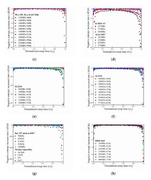
**Figure 1.** Change of the entropy increase rate with normalized creep time in the whole creep process: (a) 9Cr–1Mo steel at different temperatures; (b) 9Cr–1Mo steel under different treatment conditions (Q + T and SPWHT); (c) 9Cr–3W–3Co–1CuVNbB steel at different temperatures; (**d**–**f**) aluminum alloy at different temperatures; (g) Bar 257 steel and Ni-base super alloy at different temperatures; (h) Q460 steel at different temperatures.
