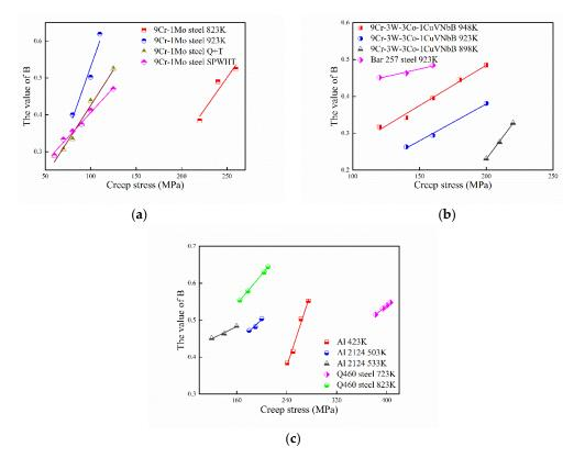
**Figure 12.** The relation between the parameter *B* and applied stress. **(a)** 9Cr-1Mo steel; **(b)** 9Cr-3W-3Co-1CuVNbB and Bar 257 steel; **(c)** Al and Q460 steel.
