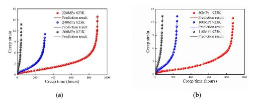
Figure 7. Prediction results of 9Cr-1Mo steel at (a) 823 K and (b) 923 K.
