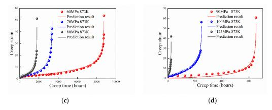
**Figure 9.** Prediction result of 9Cr-1Mo ferritic steel in quenched and tempered (Q + T) and simulated post weld heat treatment (SPWHT) conditions: (a) Q + T 60 $\sim$ 80 MPa; (b) Q + T 90 $\sim$ 125 MPa; (c) SPWHT 60 $\sim$ 80 MPa; and (d) SPWHT 90 $\sim$ 125 MPa.
