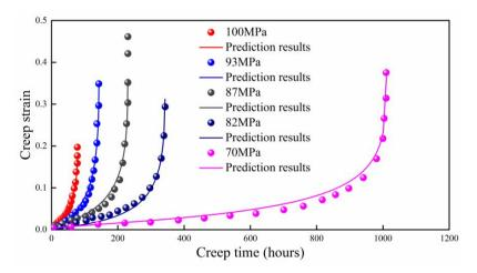
Figure 5. Prediction result of Bar 257 steel at 923 K.
